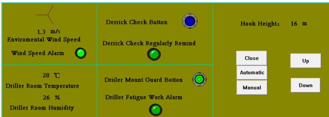
Figure 16. Configuration monitor screen of derrick and driller room.
