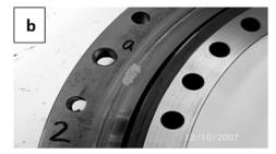
Figure 16. (a) A photo of damaged axial rollers; (b) A photo of outer raceway damage.
