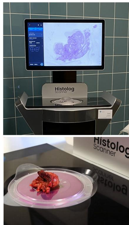
**Figure 1.** Histolog Scanner confocal imaging device (**top**) and full surgical specimen (unsliced) placed on the device for imaging (**bottom**).
