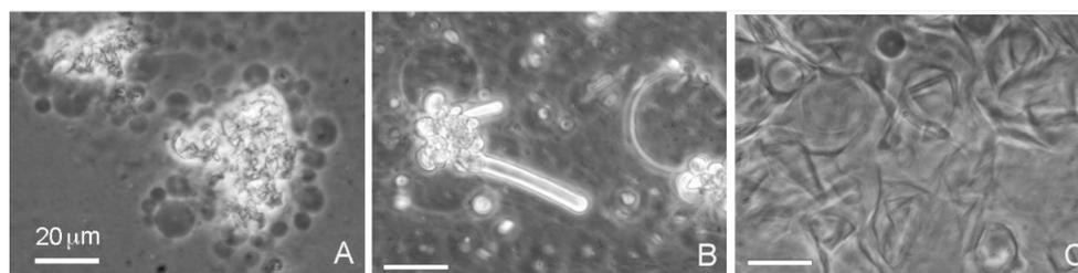
**Figure 2.** Decanoic acid (10 carbons) formed droplets at an acidic pH range (Geyser Basin sample) but partially crystallized at the alkaline pH range (Bison Pool sample) even above the transition temperature of 31 °C. All bars show 20 micrometer scales.
