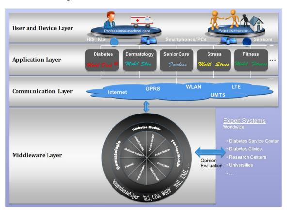
Figure 3. Architecture of the "Mobil Diab" Platform.
