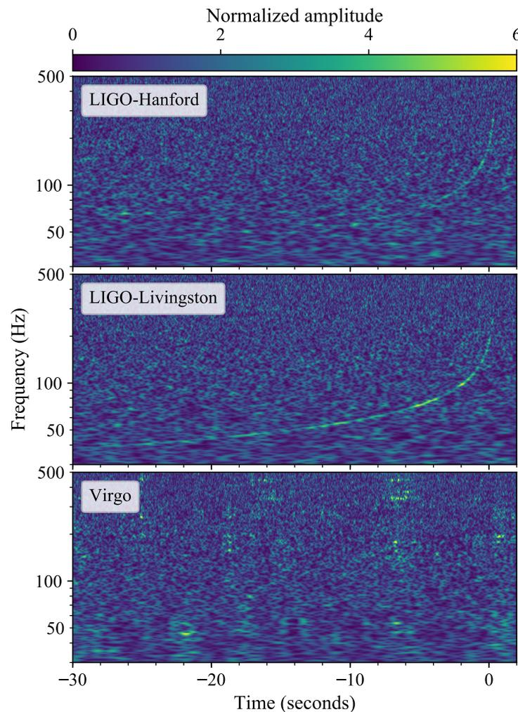
**Figure 2.** Time-frequency maps of the LIGO and Virgo detector outputs during the gravitational-wave event GW170817, created by the collision of two neutron stars. The signal stayed in the detector bandwidth for several tens of seconds, increasing in frequency following a characteristic chirp-like pattern. Graphics reproduced from [6] under Creative Commons License.
