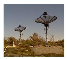
**Figure 1.** The 2.3 m radio telescopes of the Onsala Space Observatory.
