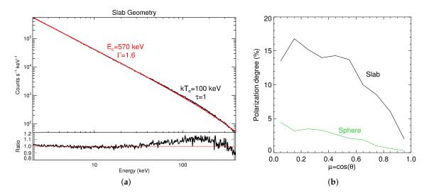
Figure 2. (a) The X-ray spectrum simulated for a slab corona with  $kT_e = 100$  keV,  $\tau = 1.0$  with Monte Carlo code for Comptonization in Astrophysics (MoCA) (in black), fitted with a power law model (in red) is shown. Residuals are reported in the bottom panel; (b) The polarization degree is plotted against the cosine of the inclination angle for two different geometries (see text for details).
