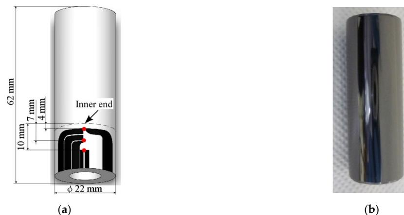
**Figure 5.** Sensor design and measuring positions: (a) measuring location 4, 7, 10 mm from inner end; (b) pressure sensor with DLC protective film.
