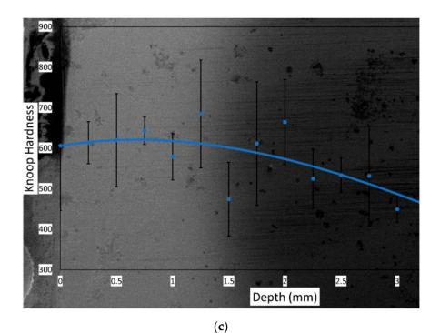
**Figure 4.** Cross-sections of (**a**) the Ni-SiC 70-30 coating, (**b**) Ni-SiC 50-50 coating, and (**c**) SiC coating with their hardness profiles overlayed to show hardness evolution into the substrate. The left side shows the coating surface in all images.
