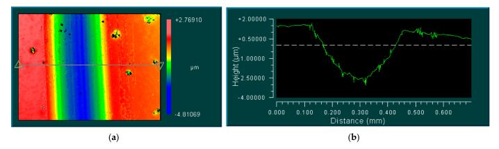
**Figure 7.** The substrate's (**a**) surface topography after the wear test and (**b**) cross-section profile at the location of the line shown in (**a**).
