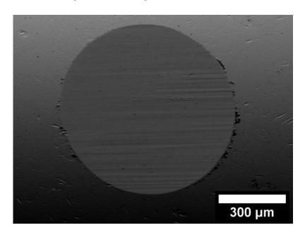
**Figure 5.** The surface of the cold-worked E52100 bearing steel ball initially used for tribotesting under SEM. The circle is a flat plane as a result of the wear the ball experienced.
