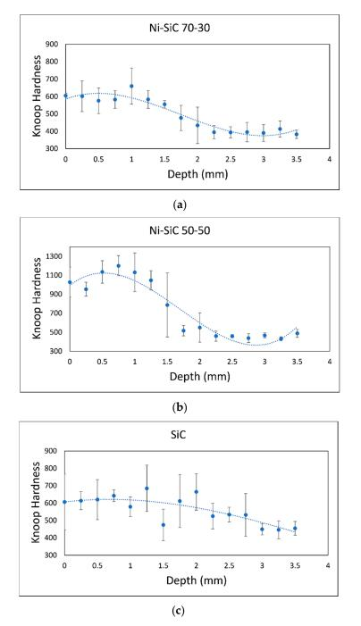
**Figure 3.** The average and standard deviation of the cross-section Knoop hardness tests for the **(a)** Ni-SiC 70-30 coating, **(b)** Ni-SiC 50-50 coating, and **(c)** SiC coating.
