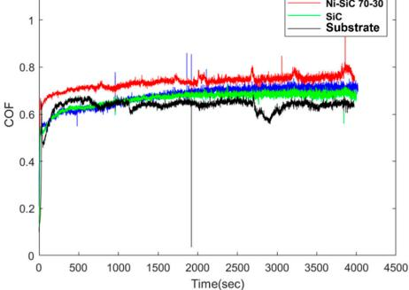
**Figure 6.** Coefficient of friction plotted against time during wear tests against an Al<sub>2</sub>O<sub>3</sub> ball counterpart for the substrate and three coatings.
