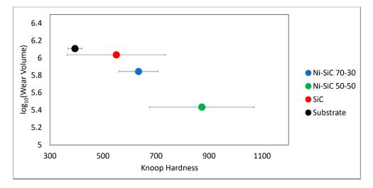
**Figure 9.** The base-10 log of the wear volume in  $\mu m^3$  versus the Knoop hardness on the surfaces of the three coatings along with the substrate.
