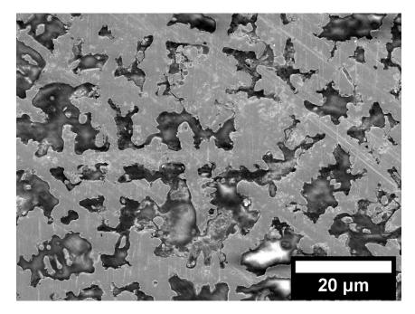
Figure 11. SEM image of the SiC coating's top surface.
