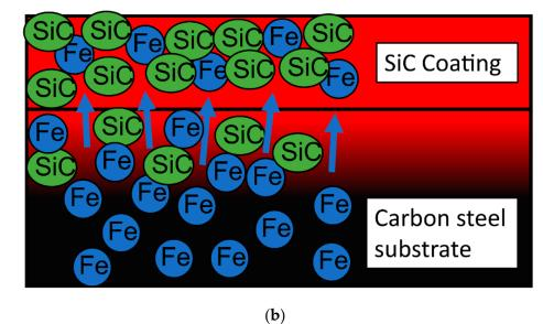
**Figure 12.** (a) An estimate of the Fe content distribution for the SiC coating and (b) the primary diffusion processes that occur in the SiC coating during Flash heating.
