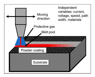
Figure 1. A schematic of the coating application process.
