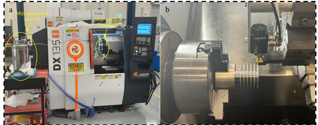
Figure 3. (a) CNC lathe and MQL setup; (b) cutting setup.
