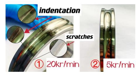
**Figure 25.** The appearance of the inner ring of the protective bearing at 20 kr/min and 5 kr/min operating conditions.
