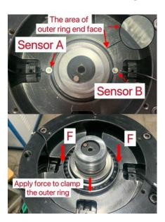
Figure 22. Installation diagram of axial collision force sensor.
