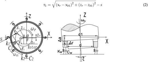
**Figure 2.** Simplified collision model of rotor and protective bearing. (a) Radial collision; (b) axial impact.
