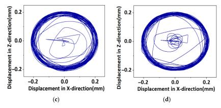
**Figure 12.** Radial displacement trajectory of non-eccentric and eccentric rotor shaft centers at different speeds. (a) 5000 r non-eccentric drop axis displacement; (b) 25,000 r non-eccentric drop axis displacement; (c) 5000 r eccentric 0.05° drop axis displacement; (d) 25,000 r eccentric 0.05° drop axis displacement.
