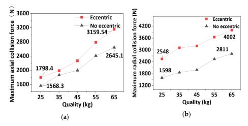
**Figure 11.** Comparison of maximum axial and radial collision forces. (**a**) Comparison of the maximum axial collision force of different quality rotor drops with an eccentricity of  $0.05^{\circ}$ ; (**b**) Comparison of the maximum radial collision force of different quality rotor drops with an eccentricity of  $0.05^{\circ}$ .
