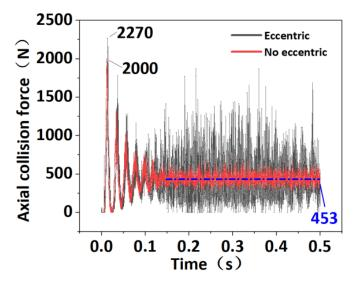
Figure 6. Comparison of the trend of the axial collision force at 0.05° with and without eccentricity.
