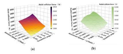
**Figure 14.** Eccentricity angle on the axial and radial collision force of rotor with different speeds. (a) Maximum axial collision force; (b) Maximum radial collision force.
