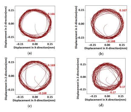
**Figure 16.** Radial axis displacement trajectory of the rotor under different axial protection gaps for non-eccentric working conditions. (a) 0.1 mm drop axis displacement; (b) 0.15 mm drop axis displacement; (c) 0.2 mm drop axis displacement.
