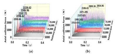
**Figure 13.** Comparison of axial collision forces between non-eccentric and eccentric rotors at different speeds. (a) Non-eccentric fall axial collision force; (b) Eccentricity 0.05° drop axial collision force.
