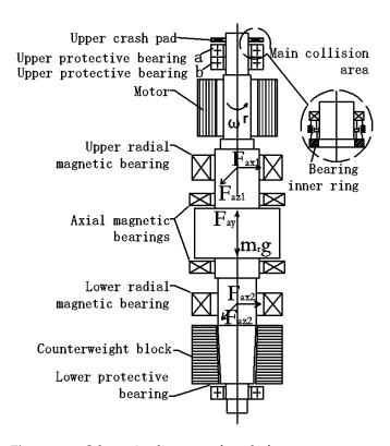
**Figure 1.** Schematic diagram of a shaft system structure of vertical magnetic levitation bearing system.
