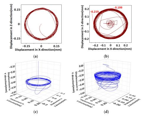
**Figure 5.** Comparison of eccentric-free and eccentric  $0.05^{\circ}$  rotor axis. (a) Non-eccentric rotor radial axial displacement; (b) Radial axial displacement of the eccentric rotor; (c) Space-wise displacement of the non-eccentric rotor axis; (d) The spatial displacement of the eccentric rotor axis.
