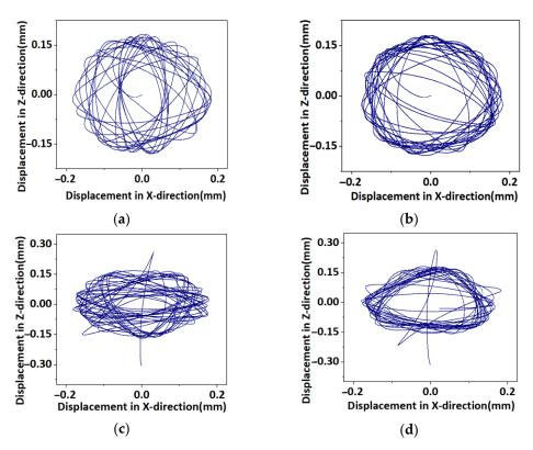
**Figure 17.** Radial axis displacement trajectory of eccentric  $0.05^{\circ}$  rotor under different axial protection clearance. (a) 0.1 mm Drop axis displacement; (b) 0.15 mm Drop axis displacement; (c) 0.2 mm Drop axis displacement; (d) 0.25 mm Drop axis displacement.
