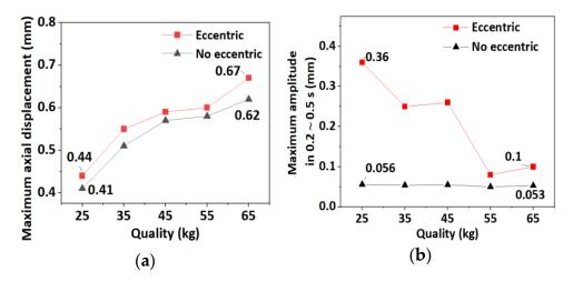
**Figure 9.** Comparison of maximum axial displacement and maximum amplitude of different quality rotor drops without eccentricity and eccentricity 0.05° working condition. (a) Comparison of the maximum axial displacement; (b) Comparison of the maximum amplitude within the 0.2~0.5 s.
