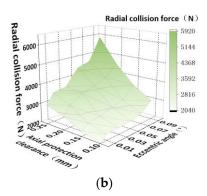
**Figure 18.** Eccentricity angle on the axial and radial collision forces of rotor drops with different axial clearances. (a) Maximum axial collision force; (b) Maximum radial collision force.
