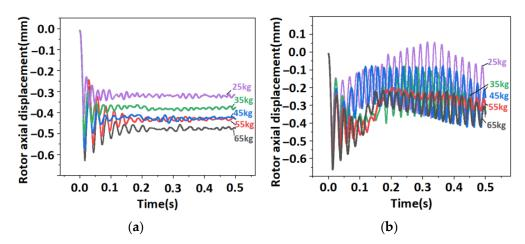
**Figure 8.** Comparison of non-eccentric and eccentric  $0.05^{\circ}$  rotor radial collision force. (a) Axial displacement of the rotor drops of different qualities under non-eccentric working conditions. (b) Axial displacement of rotor drops of different qualities at  $0.05^{\circ}$  eccentric conditions.
