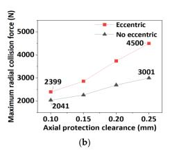
**Figure 19.** Comparison of maximum axial and radial collision forces under non-eccentric and eccentric working conditions. (a) Comparison of the maximum axial collision force of different axial protection clearance rotor drops under the 0.05° eccentric working condition; (b) Comparison of the maximum radial collision force of different axial protection gap rotor drops under the 0.05° eccentric working condition.
