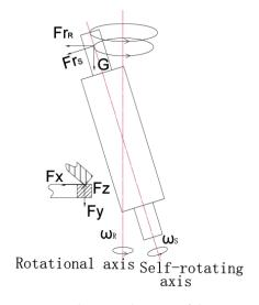
Figure 4. Schematic diagram of the rotor simplified model under eccentric working conditions.
