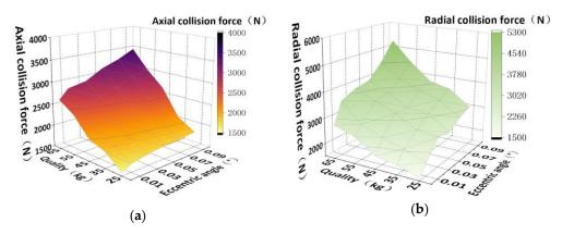
**Figure 10.** Axial and radial collision forces of quality on rotors with different speeds. (a) Maximum axial collision force; (b) Maximum radial collision force.
