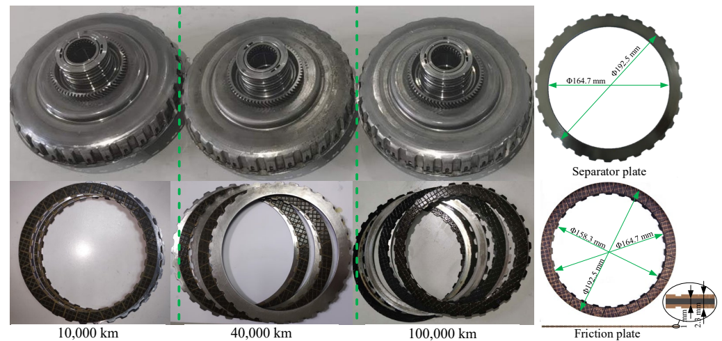
Figure 3. Wet clutches with different service mileages.
