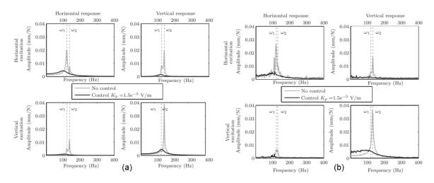
**Figure 2.** Theoretical and experimental frequency response of the rotating disc due to impulse excitations where the hybrid lubrication is illustrated in gray and the active lubrication in black: (a) theoretical results and (b) experimental results [39].
