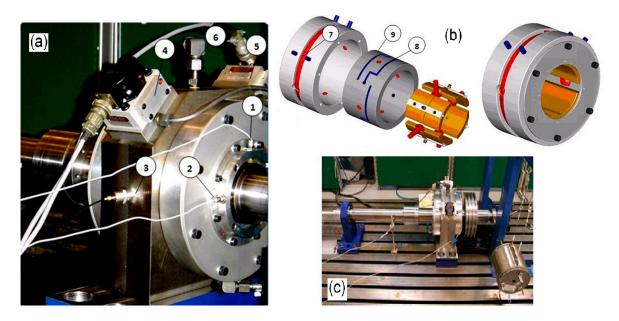
**Figure 3.** (a) Sliding bearing with incorporated sensing and actuation systems; (b) design solution and compactness; (c) test bench composed of a flexible rotor-disc excited by an electromagnetic shaker and controlled via active sliding bearing.
