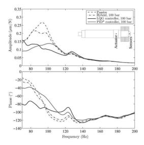
**Figure 4.** Horizontal and vertical lateral dynamics of the rotor–bearing system measured at the end of the shaft and excited by the electromagnetic shaker when four cases are investigated: hydrodynamic (conventional); hybrid using 100 bar; active using a LQG model-based controller; and active using an empirically-tuned PID controller [43]. Copyright from Elsevier.
