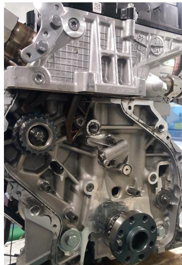
Figure 12. The deactivated timing drive system.
