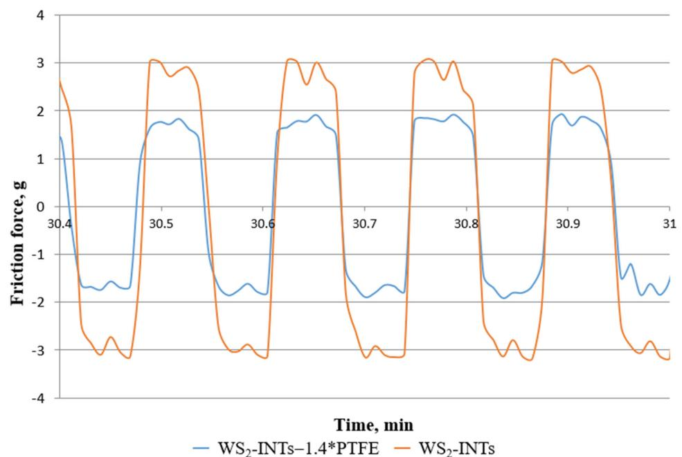
Figure 4. Typical variation of the friction force under a steady friction state of WS<sub>2</sub>-INTs (red) and WS<sub>2</sub>-INTs—1.4\*PTFE (blue; significantly smaller variation).
