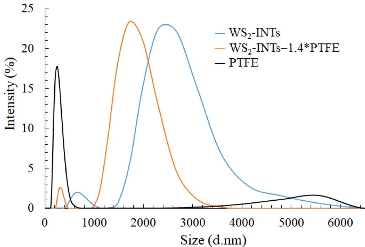
**Figure 2.** DLS size distribution histograms of the PTFE preparation, WS<sub>2</sub>-INTs, and WS<sub>2</sub>-INTs—1.4\*PTFE.
