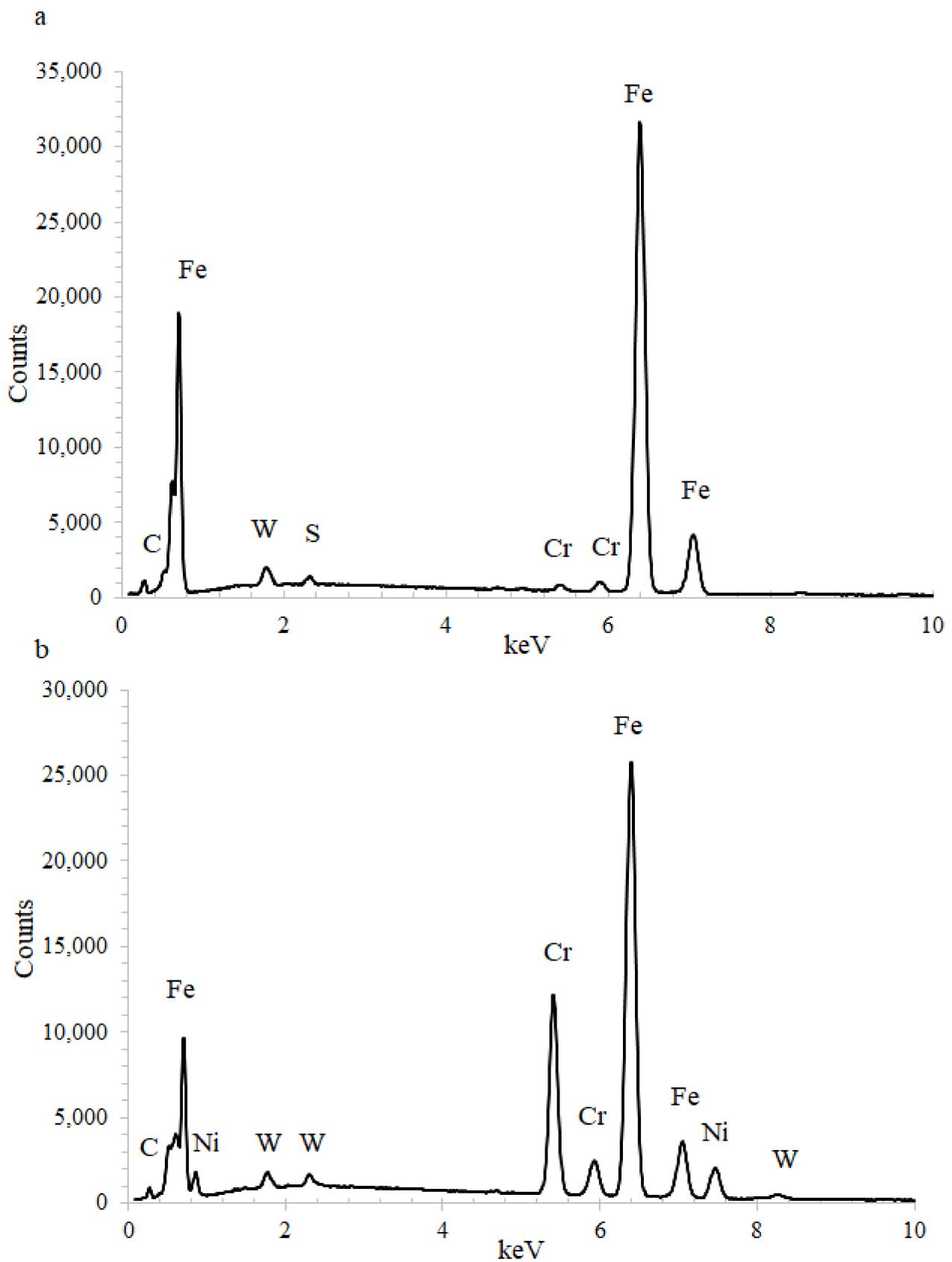
**Figure 8.** EDS spectra from the wear track (a) and wear spot on the ball surface (b) after the friction test in PAO4 + 1% WS<sub>2</sub>-INTs—1.4\*PTFE.
