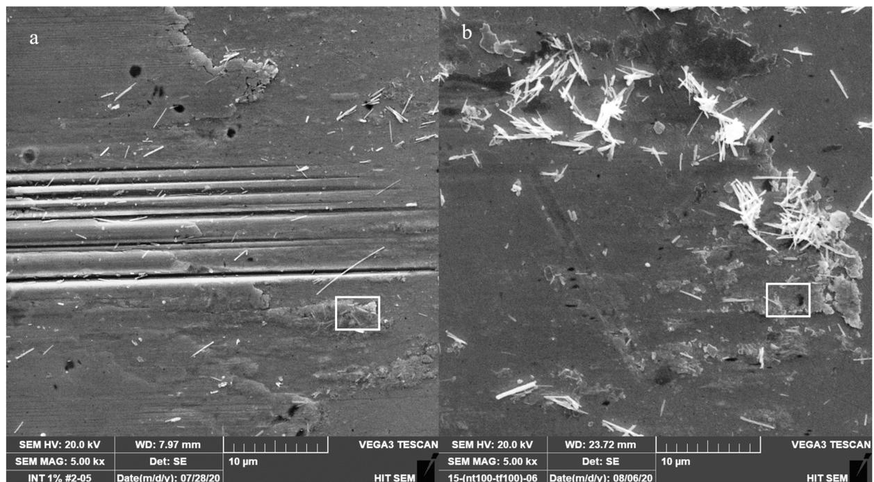
**Figure 7.** High magnification SEM images of wear spots on the surface of the ball after friction in PAO4 oil supplemented by 1% of either (a) WS<sub>2</sub>-INTs (a) or (b) WS<sub>2</sub>-INTs—1.4\*PTFE. Rectangles depict locations of EDS measurements. Some agglomeration of WS<sub>2</sub>-INTs is observed around the contact spots, in particular in (b).
