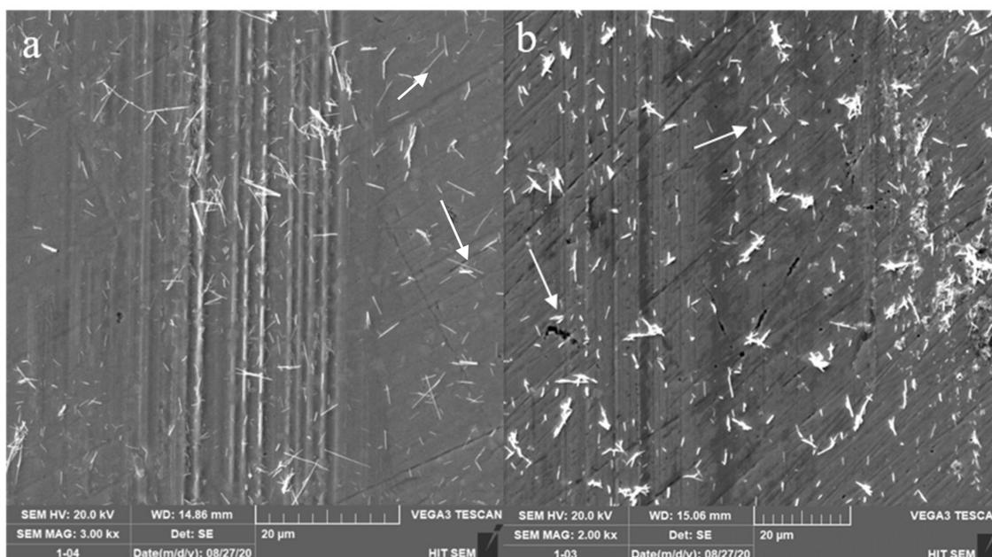
**Figure 5.** SEM images of wear tracks on the surface of plates lubricated by (a) PAO4 – 1% WS<sub>2</sub>-INTs and (b) PAO4 + 1% WS<sub>2</sub>-INTs—1.4\*PTFE.
