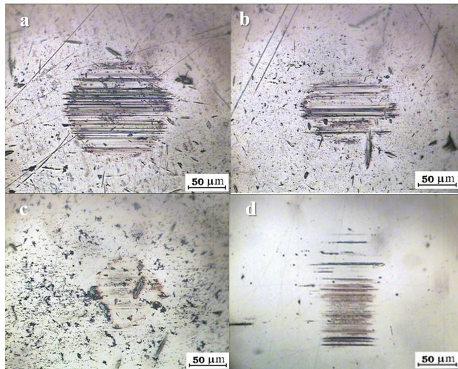
**Figure 6.** Optical microscopy images of wear spots on the surface of balls rubbed with synthetic PAO4 oil (a) or with 1% of WS<sub>2</sub>-INTs (b), WS<sub>2</sub>-INTs—1.4\*PTFE (c), or WS<sub>2</sub>-INTs—5.6\*PTFE (d).
