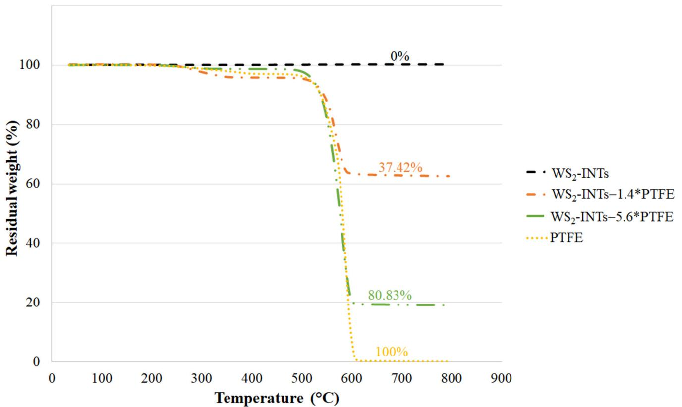
Figure 3. TGA analysis of WS<sub>2</sub>-INTs—weight loss percentage appears near each thermogram.
