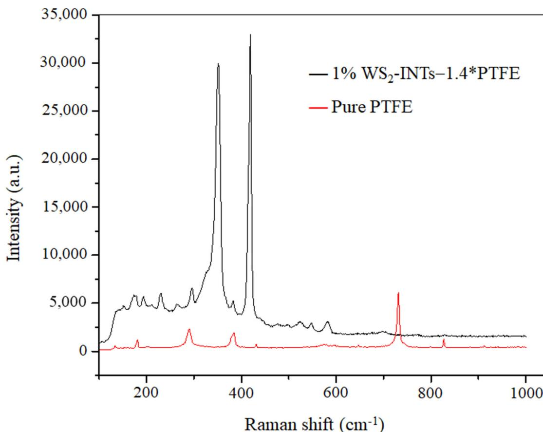
Figure 9. Micro-Raman spectra of pure PTFE and 1% WS<sub>2</sub>-INTs—1.4\*PTFE after friction in PAO4.
