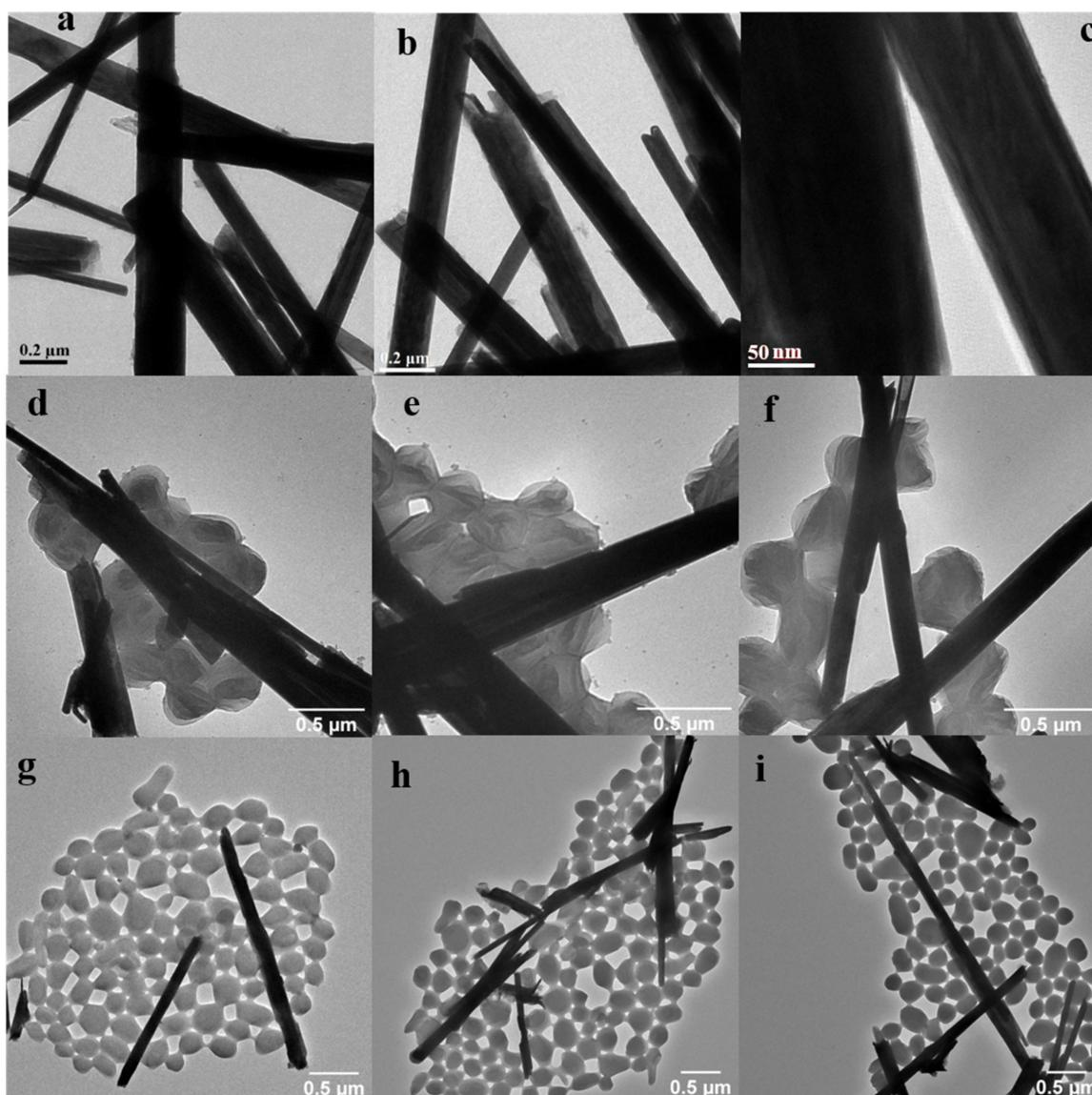
**Figure 1.** TEM images of (a–c) WS<sub>2</sub>-INTs; (d–f) WS<sub>2</sub>-INTs—1.4\*PTFE; (g–i) WS<sub>2</sub>-INTs—5.6\*PTFE.
