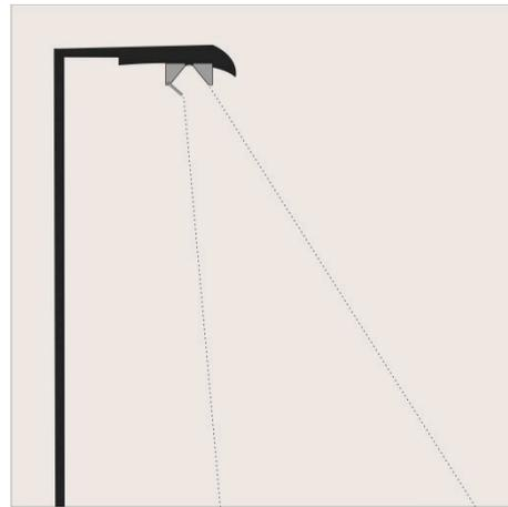
**Figure 1.** Design of an insect-friendly road luminaire. Mast arm is matt black to reduce reflection. The light point overhang from the center of the luminous area is 1.0 m without any slope. The road lighting design aims at a strict light distribution curve with a luminous intensity of 0 cd in the non-target area. Illustrated by Pérez-Vega.
