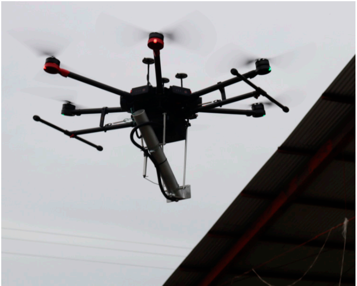
Supplementary Figure S5. Aerial release of Aedes aegypti sterile males from the tube device attached to the drone in flight.
