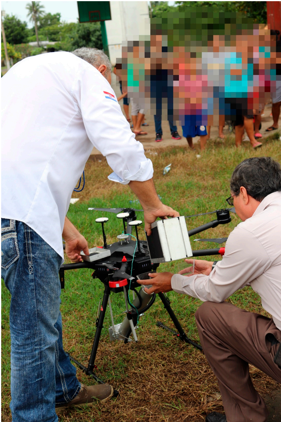
Supplementary Figure S4. Loading sterile males of Aedes aegypti into the release device attached to the aerial drone immediately prior to release.
