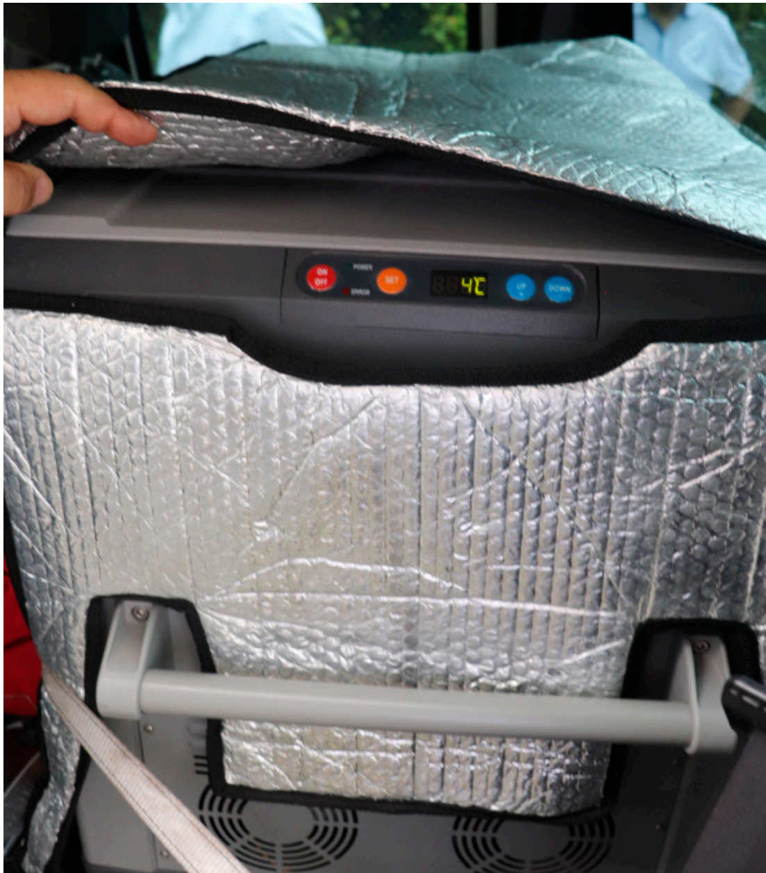
Supplementary Figure S3. Portable refrigeration unit used to transport Aedes aegypti sterile males from the production laboratory to the field site.
