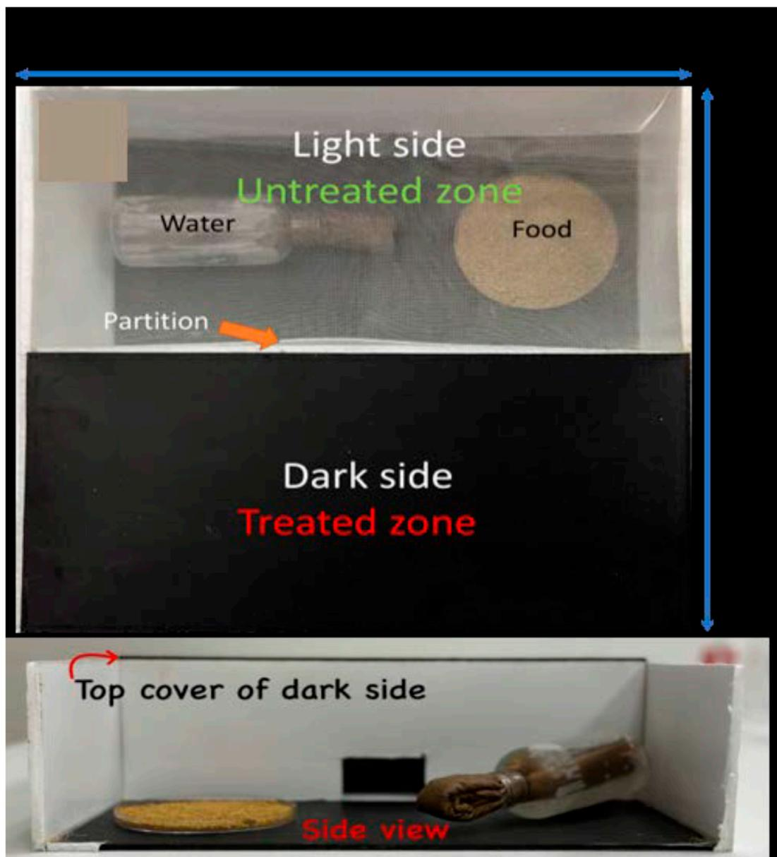
**Figure 2.** Modified Ebeling choice box to test the performance of insecticide-based paints. The flooring of dark areas received 20.5 mg of deltamethrin, 41 mg of transfluthrin, or 57.4 mg of alphacypermethrin. Cockroaches were released in the lighted area and allowed to move freely through a window located in the lower part of the dividing wall. Cockroaches were continuously exposed to the treated bottoms of the dark halves because they are unable to climb smooth vertical surfaces.
