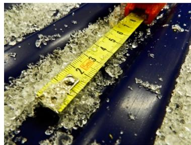
**Figure 2.** The sintered and granulated snow used for the tests.
