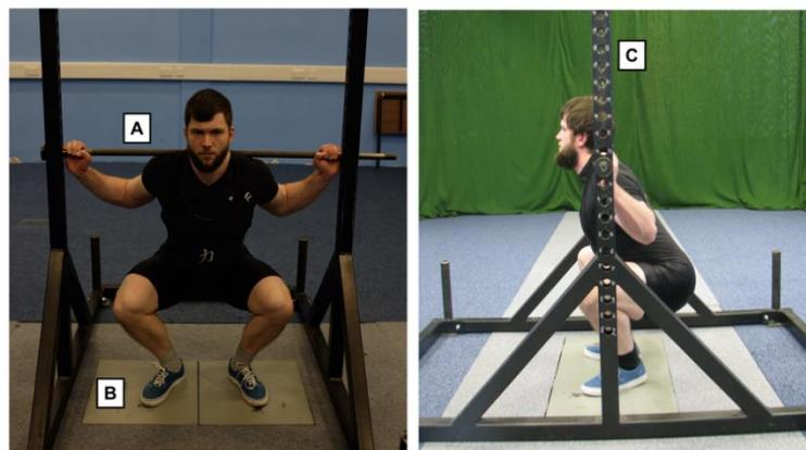
**Figure 1.** Isometric squat rack apparatus and subject setup: (left) = front view, (right) = side view. A = fixed barbell, B = AMTI force plates, C = adjustable bar heights (2.5 cm between rack heights). In this example, the isometric squat was performed with knee and hip angles of  $65^\circ$  and  $115^\circ$ , respectively.
