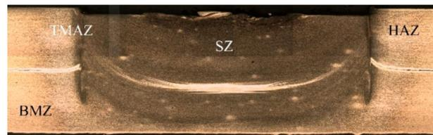
Figure 3. Cross-section of the RFSSW joint.
