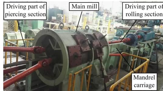
**Figure 2.** TSR testing mill.
