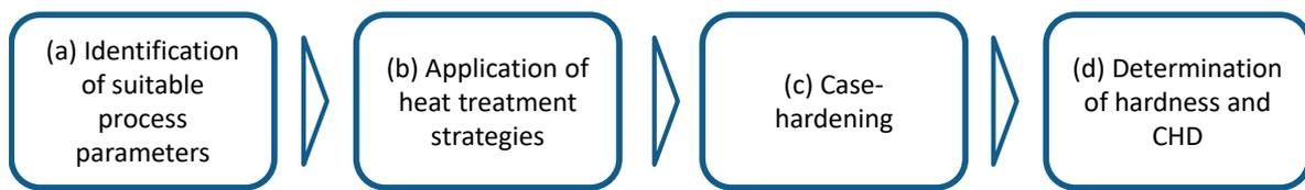
**Figure 2.** Experimental approach for the investigation of case-hardening behavior of additively manufactured 16MnCr5.
