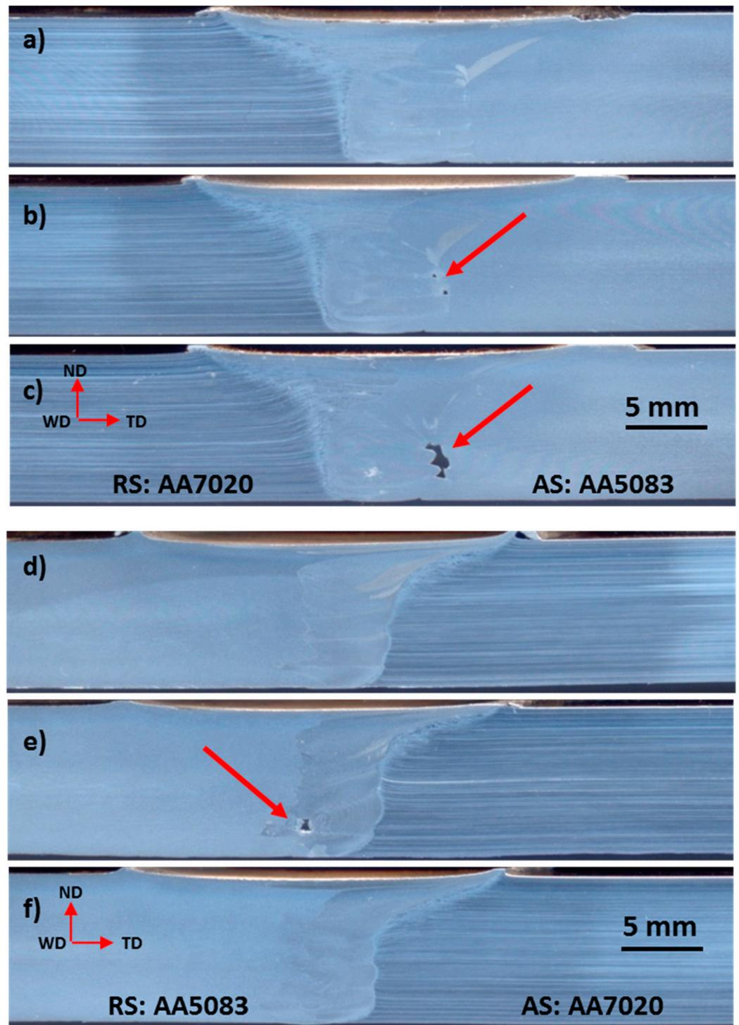
**Figure 8.** Cross sections of friction stir welded joints at different rotational and traverse speeds for AA5083/AA7020 and AA7020/AA5083 after etching: (a,d) 500 rpm, 20 mm/min, (b,e) 500 rpm, 40 mm/min and (c,f) 500 rpm, 80 mm/min.
