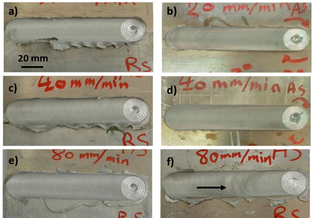
**Figure 6.** Surface appearance of friction stir welded joints AA5083/AA7020 at different rotation and traverse speeds: (a) AA5083/AA7020, 500 rpm, 20 mm/min, (b) AA7020/AA5083, 500 rpm, 20 mm/min, (c) AA5083/AA7020, 500 rpm, 40 mm/min, (d) AA7020/AA5083, 500 rpm, 40 mm/min, (e) AA5083/AA7020, 500 rpm, 80 mm/min and (f) AA7020/AA5083, 500 rpm, 80 mm/min.
