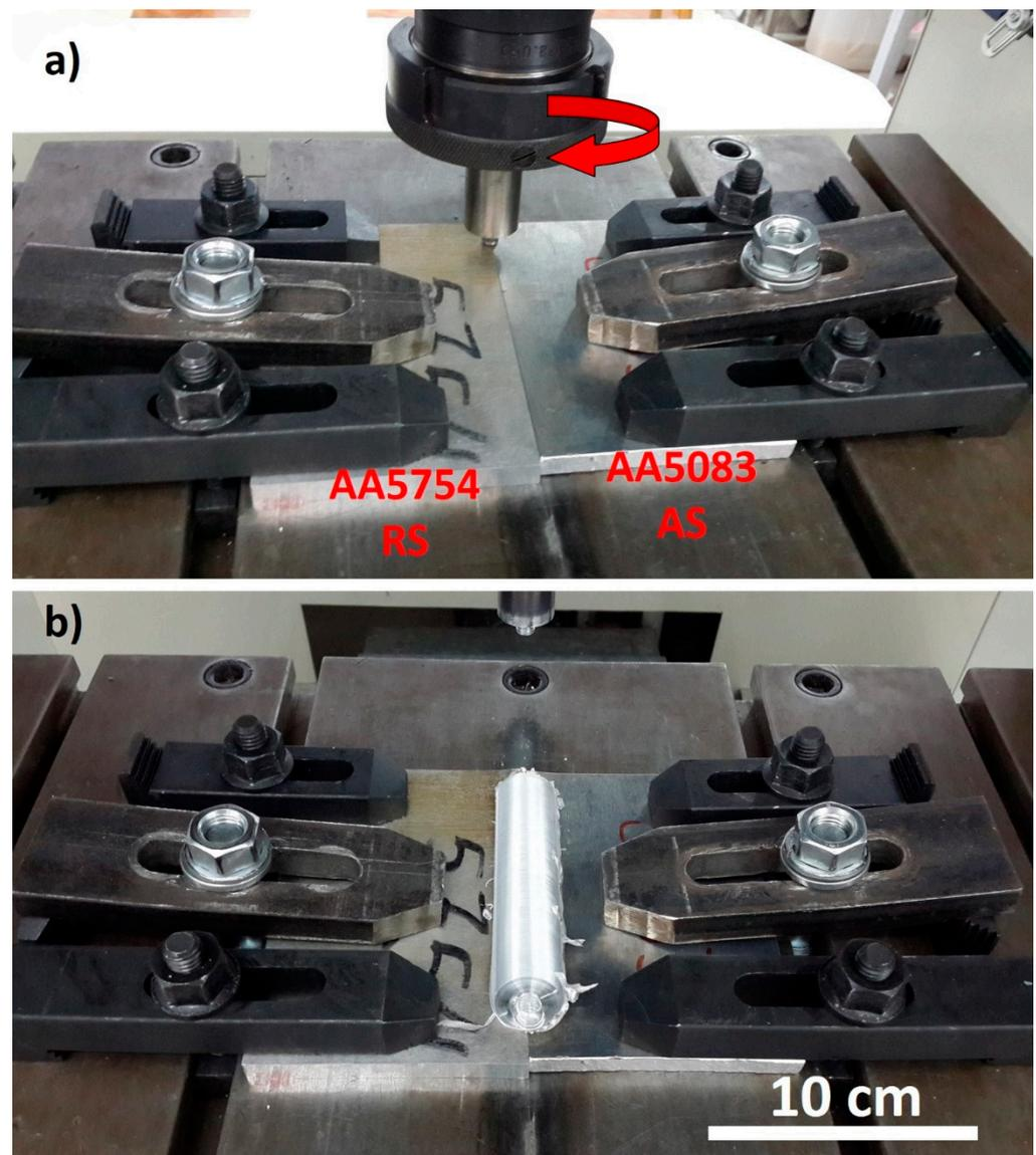
**Figure 2.** (a) The clamping of the plates on the FSW machine table with the advancing side (AS) and retreating side (RS) indicated and the tool rotation direction indicated also by the red arrow and (b) Aluminum alloys butt joint on the table after FSW.
