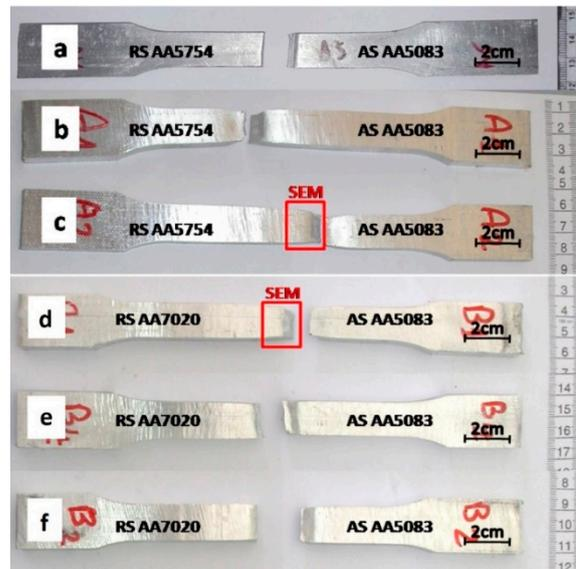
**Figure 12.** Fracture locations of tensile test specimens of AA5083/AA5754 joints at different welding parameters: (a) 400 rpm–20 mm/min, (b) 400 rpm–40 mm/min and (c) 400 rpm–60 mm/min and fracture locations of AA5083/AA7020 joints at 500 rpm but different travel speeds and positions; (d) AA7020 AS-20 mm/min, (e) AA7020 AS-40 mm/min and (f) AA7020 AS-80 mm/min.
