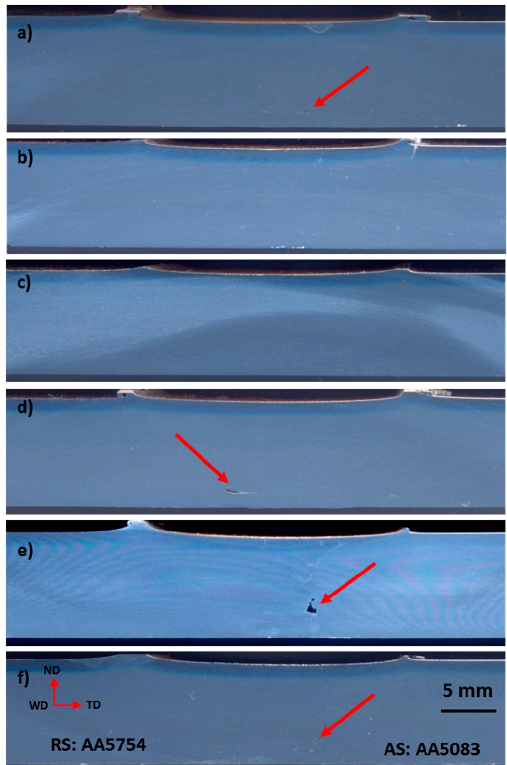
**Figure 7.** Polishing cross-sections of friction stir welded joints AA5083/AA5754 at different rotational and traverse speeds. Arrows refer to the tunnel defects: (a) 400 rpm, 20 mm/min, (b) 400 rpm, 40 mm/min, (c) 400 rpm, 60 mm/min, (d) 600 rpm, 20 mm/min, (e) 600 rpm, 40 mm/min and (f) 600 rpm, 60 mm/min.
