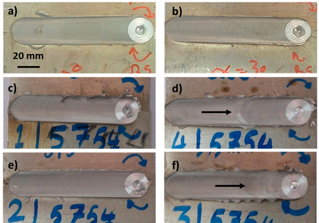
**Figure 5.** Surface appearance of friction stir welded AA5083/AA5754 joints at different rotation and traverse speeds: (a) 400 rpm, 20 mm/min, (b) 600 rpm, 20 mm/min, (c) 400 rpm, 40 mm/min, (d) 600 rpm, 40 mm/min, (e) 400 rpm, 60 mm/min and (f) 600 rpm, 60 mm/min.
