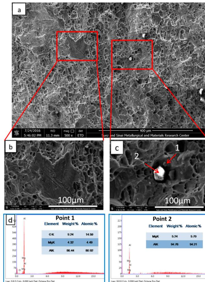
**Figure 13.** SEM micrographs of the fracture surface of tensile test sample of AA5083/AA5754 joint at 400 rpm–60 mm/min, (a) mixed fracture mode (b) brittle fracture features, (c) ductile fracture features, (d) EDX spot analysis of the points 1 and 2.
