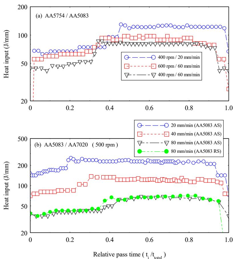
**Figure 4.** Calculated heat input of friction stir welded joints at different rotation and traverse speeds (i.e., at different  $\omega/v$  ratios) versus the relative pass time ( $t_1/t_{total}$ ) for FSW for the joints (a) AA5083/AA5754 and (b) AA5754/AA7020.
