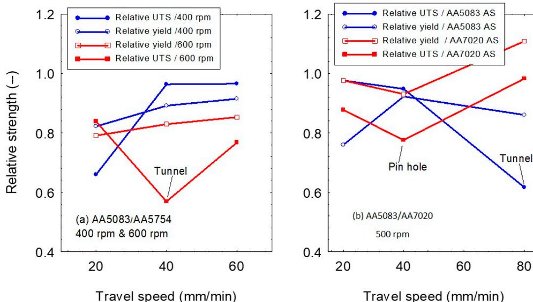
**Figure 11.** Relative tensile strength ( $\sigma_{UTS}$  joint/ $\sigma_{UTS}$  5083) and relative yield stress ( $\sigma_{0.2\%}$  joint/ $\sigma_{0.2\%}$  5083) of the produced FSW joints against the welding speeds.
