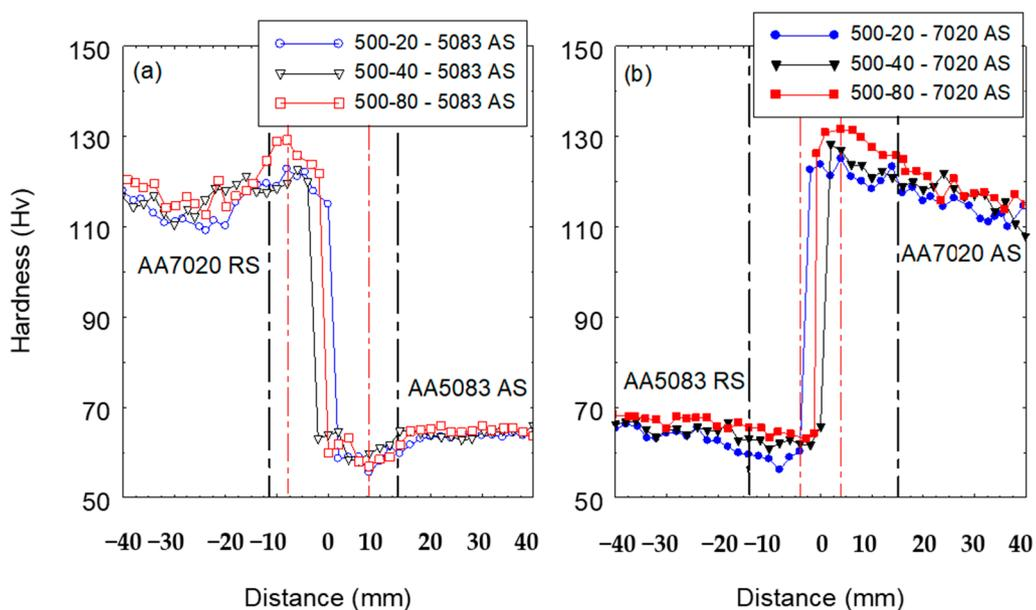
**Figure 10.** Hardness distribution across the joints (a) AA5083/AA7020 and (b) AA7020/AA5083 welded at travel speeds of 20, 40 and 80 mm/min showing the effect of the joint arrangement.
