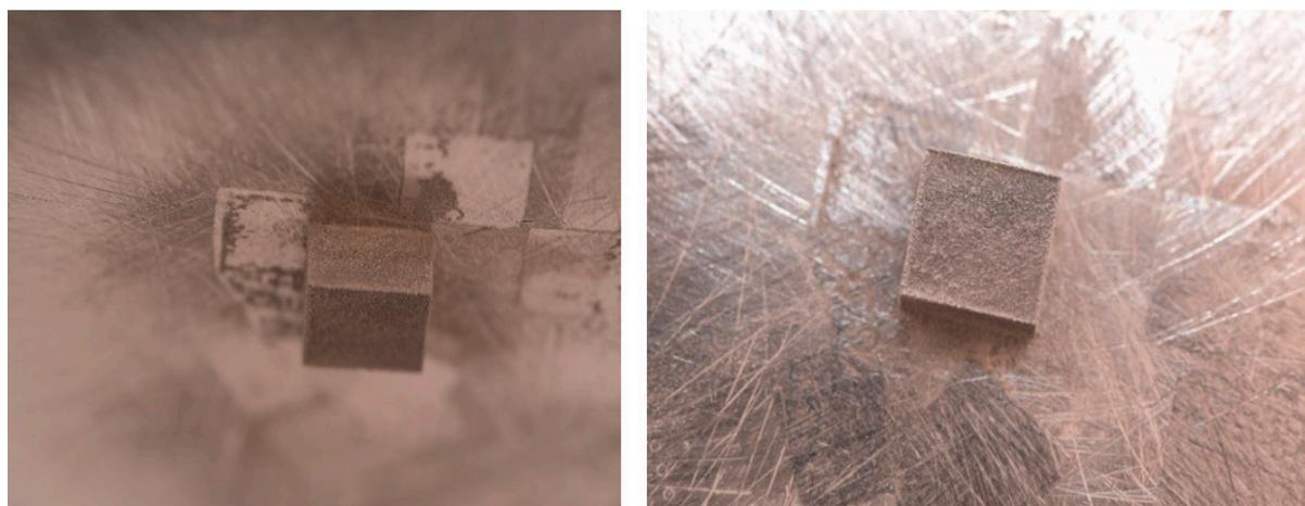
**Figure 14.** The sample of Mg-10Zn-0.8Ca-0.5Zr alloy-powder processed by SLM—two macro images of the same sample.
