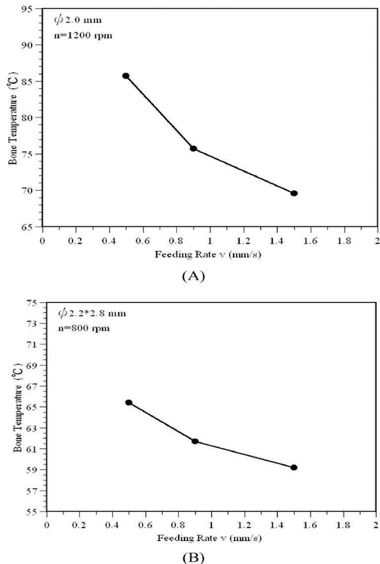
**Figure 10.** Maximum temperature decreases as the feed rate using two types of drills: (A) pilot drill, (B) twist drill [37].
