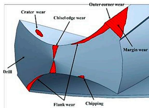
Figure 8. Drill bit wear [78].
