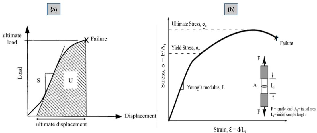
Figure 4. (a) Load-displacement curve; (b) tensile stress–strain curve of bone [21].
