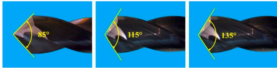
**Figure 13.** Drill bit point angles [109].
