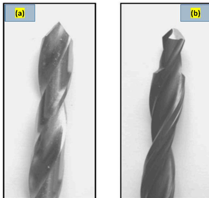
**Figure 12.** Standard surgical (a) twist drill; (b) two-step drill.
