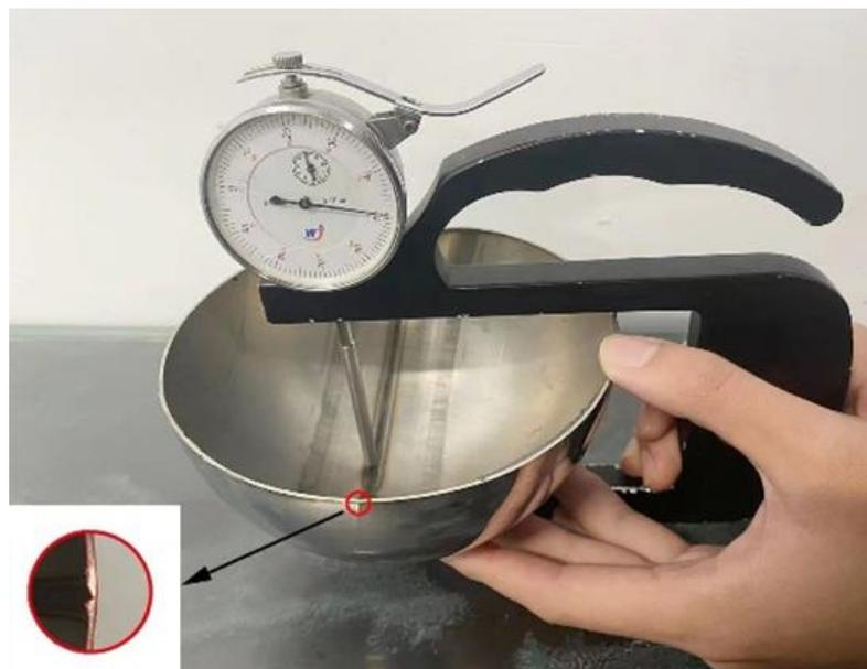
**Figure 6.** Welding thickness measurement.
