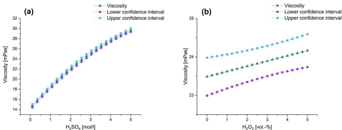
**Figure 6.** Viscosity dependency on the concentration of (a) the leaching medium (H<sub>2</sub>SO<sub>4</sub>) and (b) the reducing agent (H<sub>2</sub>O<sub>2</sub>) with parameters at otherwise average values (60 °C, 75 g/L solids, 240 min), confidence interval of 95%.
