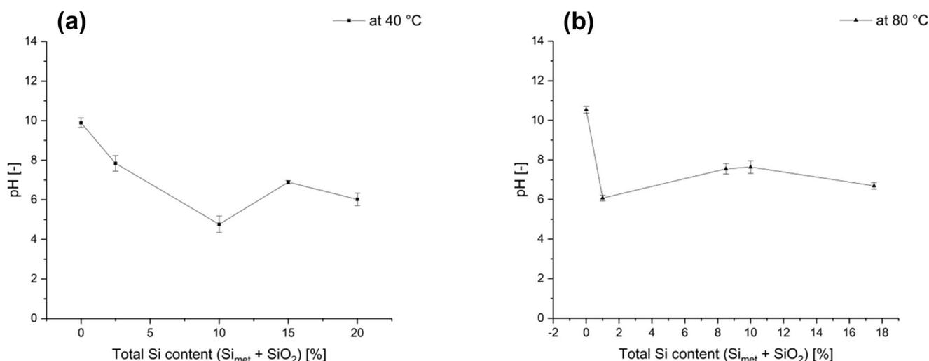
**Figure 5.** pH of the solutions after the end of leaching (0.5 M  $\text{H}_2\text{SO}_4$ ) at (a) 40 °C and (b) 80 °C as a function of the total amount of silicon ( $\text{SiO}_2 + \text{Si}_{\text{met}}$ ) added.
