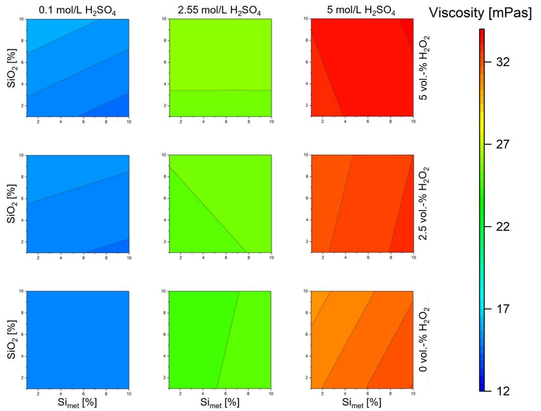
**Figure 9.** 4D contour plot for the change in viscosity as a function of  $Si_{met}$ ,  $SiO_2$ ,  $H_2SO_4$  and  $H_2O_2$  concentration in the leaching solution at an S/L ratio of 100 g/L and a leaching temperature of 80 °C.
