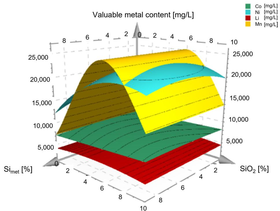
**Figure 13.** Surface plots for Ni, Co, Li and Mn leaching and their dependencies on the SiO<sub>2</sub> and Si<sub>met</sub> content of the leaching solution.
