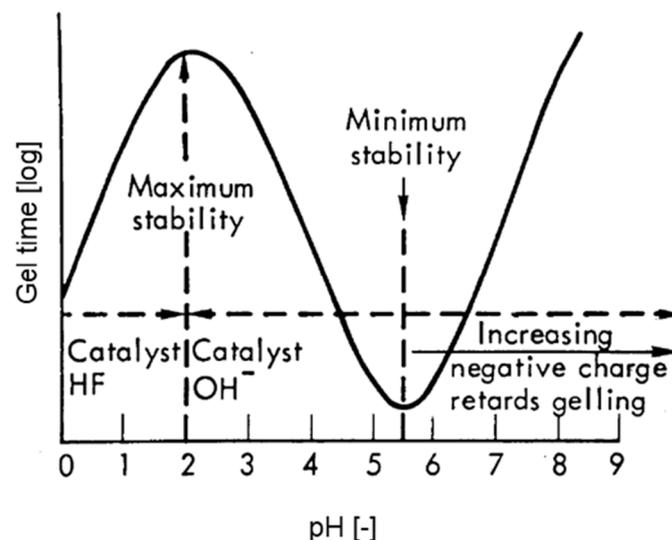
**Figure 3.** Dependence of gel time on pH in the absence of salts for Si sol stability, reprinted with permission from Ref. [1].
