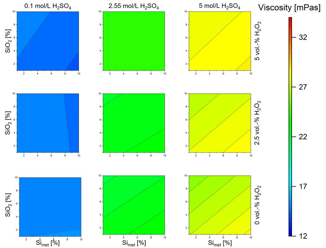
**Figure 7.** 4D contour plot for the change in viscosity as a function of  $Si_{met}$ ,  $SiO_2$ ,  $H_2SO_4$  and  $H_2O_2$  concentration in the leaching solution at an S/L ratio of 50 g/L and a leaching temperature of 40 °C.
