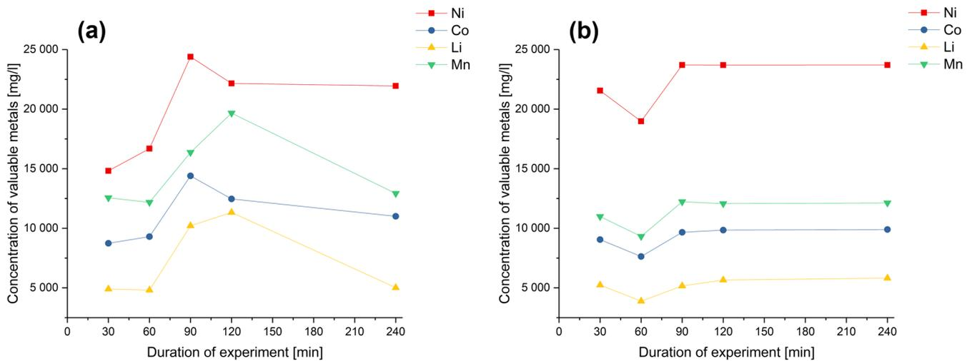
**Figure 12.** Concentration curve of Ni, Co, Li and Mn in the leaching solutions as a function of the leaching time in comparison with the results at (a) 0% and (b) 20% Si<sub>met</sub> and SiO<sub>2</sub> (in total) with otherwise constant parameters (5 mol/L H<sub>2</sub>SO<sub>4</sub>, 80 °C, 100 g/L solids, 0% H<sub>2</sub>O<sub>2</sub>).
