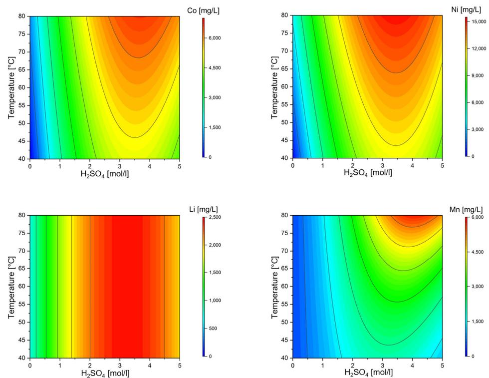
**Figure 11.** Contour plot of the statistical test evaluation for the leached fractions of Co, Ni, Li and Mn without the addition of Si<sub>met</sub>, SiO<sub>2</sub> or H<sub>2</sub>O<sub>2</sub> as a function of temperature and H<sub>2</sub>SO<sub>4</sub> concentration.
