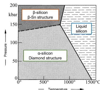
**Figure 1.** States of silicon with dependence on pressure and temperature, adapted with permission from Ref. [1].
