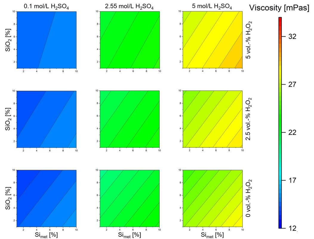
**Figure 8.** 4D contour plot for the change in viscosity as a function of  $Si_{met}$ ,  $SiO_2$ ,  $H_2SO_4$  and  $H_2O_2$  concentration in the leaching solution at an S/L ratio of 50 g/L and a leaching temperature of 80 °C.
