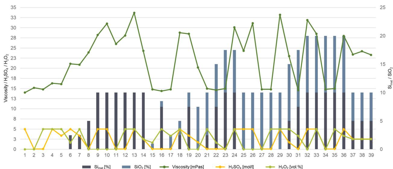
**Figure 4.** Results of the viscosity [mPas] determination of solutions 1 to 39 as a function of  $\text{H}_2\text{SO}_4$  [mol/L] and  $\text{H}_2\text{O}_2$  [vol.-%] concentration as well as the amount of  $\text{SiO}_2$  and  $\text{Si}_{\text{met}}$  [mass-% of black mass] added to the solution.
