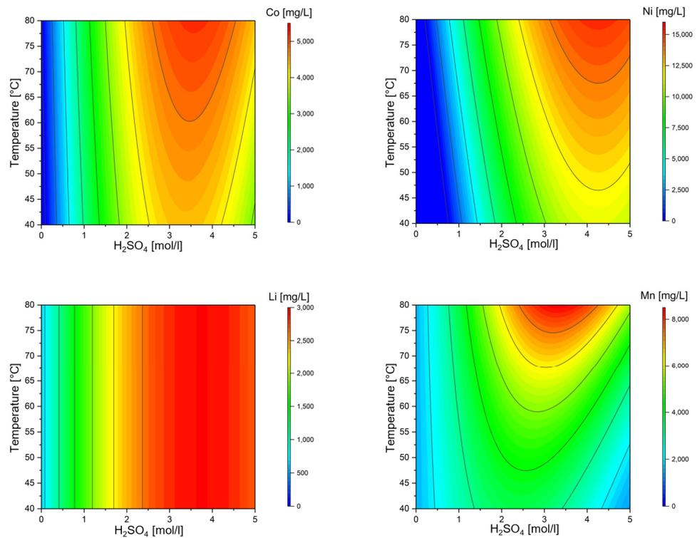
**Figure 10.** Contour plot of the statistical test evaluation for the leached fractions of Co, Ni, Li and Mn with addition of the maximum amount of  $Si_{met}$  and  $SiO_2$  without the application of  $H_2O_2$  and an S/L ratio of 50 g/L as a function of temperature and  $H_2SO_4$  concentration.
