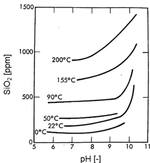
**Figure 2.** Dependence of  $\text{SiO}_2$  solubility on temperature for amorphous silica, reprinted with permission from Ref. [1].
