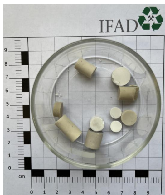
Figure S2. Sample sintered LLZO #2 before grinding.
