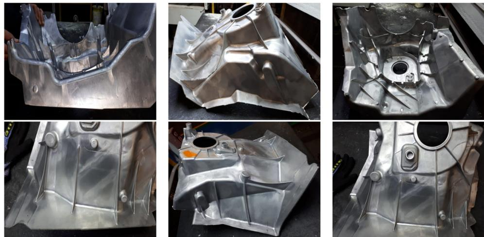
**Figure 9.** Results of blister test, none of the casting had an air trap.
