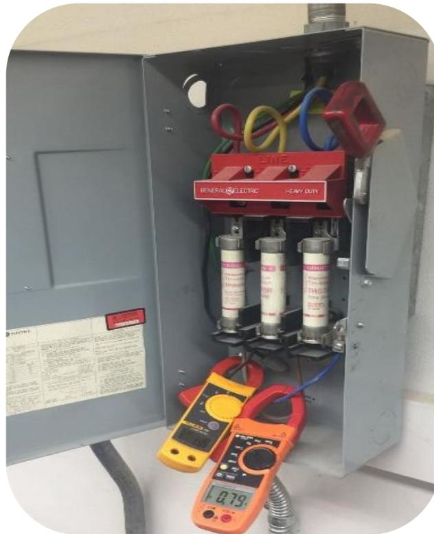
**Figure 5.** Test rig for power consumption measurement.
