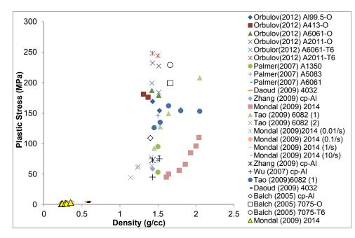
Some syntactic foam composites are found to have less than 0.4 g/cc density in Figure 9. These data points belong to foams that contain fly ash cenospheres as well as matrix porosity to create a hybrid foam structure. Such foams are found to have very low strength compared to syntactic foams containing porosity only inside hollow particles.
