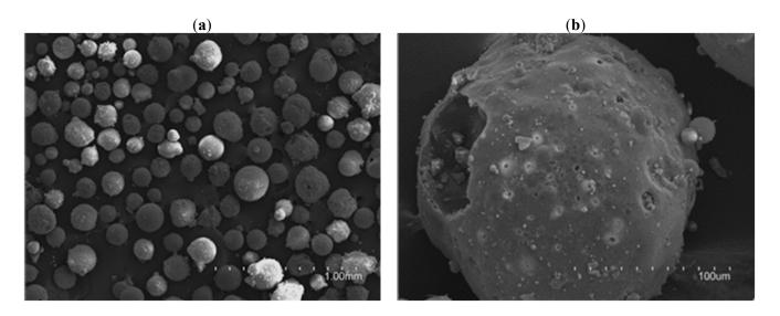
Hollow particles of alumina, silica, and silicon carbide have been used in some studies on MMSFs. An example of alumina hollow particles is shown in Figure 3a. High surface area of such particles (observed in Figure 3b) can provide advantage in improving interfacial bonding with the matrix material and result in strong bonding.
