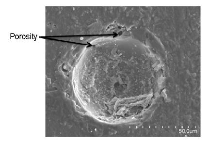
Cenospheres are primarily composed of SiO<sub>2</sub> and Al<sub>2</sub>O<sub>3</sub>. Silicon tends to react at the interface with magnesium present in the matrix and form Mg<sub>2</sub>Si and MgO. Thermodynamic calculations show that MgAl<sub>2</sub>O<sub>3</sub> may also generate, but it reacts with magnesium and decomposes into MgO and Al.
