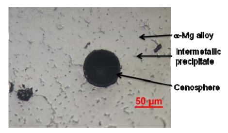
**Figure 7.** Scanning electron micrograph of AZ91D/fly ash cenosphere composite, where porosity and defects are visible in the cenosphere shell.
