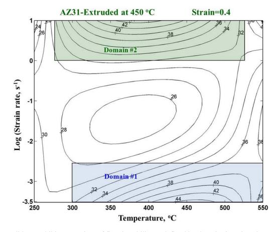
Figure 11. Processing map obtained at a strain of 0.4 for AZ31 magnesium alloy extruded at 450 °C.
