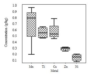
Figure 1. Statistics of Mn, Ti, Cu, Zn and Ni content in EMHS.
