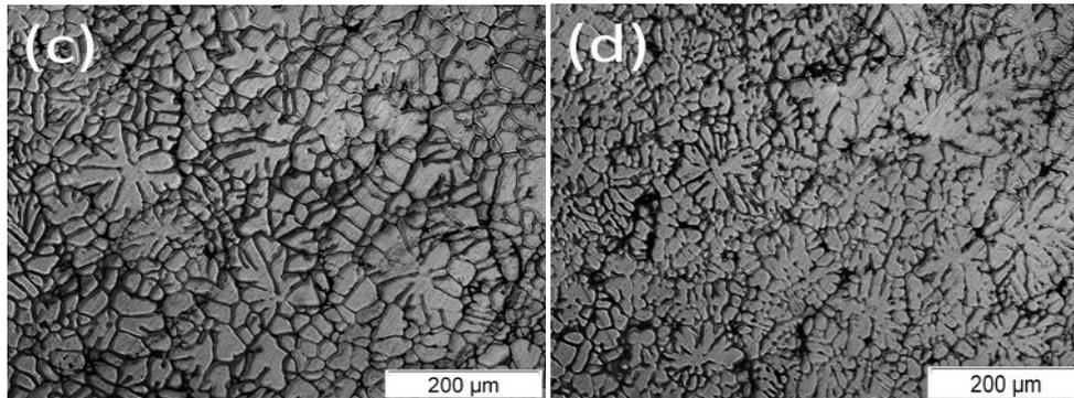
These micrographs show that the microstructures prepared under higher applied pressures are much finer and smaller  $\alpha$ -primary dendrites. It is clear that the squeezing pressure has significant influence on the microstructure of the alloy [7]. Furthermore, the inter-metallic phases in the alloy with no applied pressure are coarser than those under high squeezing pressure. This effect is a result of the change in phase diagram according to the Clausius-Clapeyron Equation [6]:
