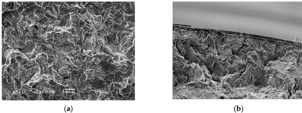
**Figure 6.** Hydrogen-assisted micro-damage (TTS) in wires after CERT tests: (a) hot rolled steel, speed type 1 (Figure 4a); (b) prestressing steel, speed type 2 (Figure 5c).
