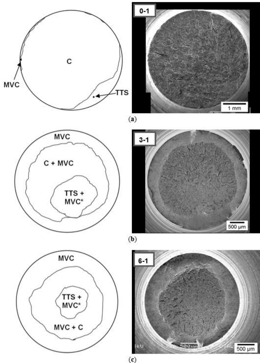
**Figure 4.** Micro-fracture maps (MFMs) for low loading rate (crosshead speed type 1 of 0.001 mm/min): (a) hot rolled steel (base material that is not cold drawn at all); (b) three drawing steps; (c) six drawing steps (heavily-drawn commercial prestressing steel).
