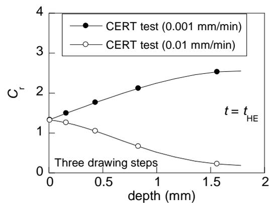
**Figure 9.** Radial distribution of relative hydrogen concentration for both loading rates at the instant of final failure during a CERT test ( $t = t_{HE}$ ) of a steel undergoing three steps of cold drawing. Depth is defined in radial direction from the notch tip.
