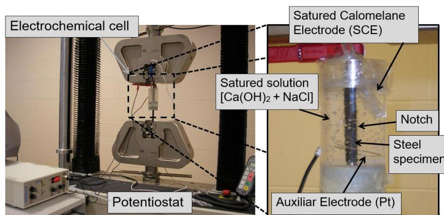
**Figure 3.** Constant extension rate tensile (CERT) test under cathodic electrochemical conditions including a detailed view of the electrochemical cell.
