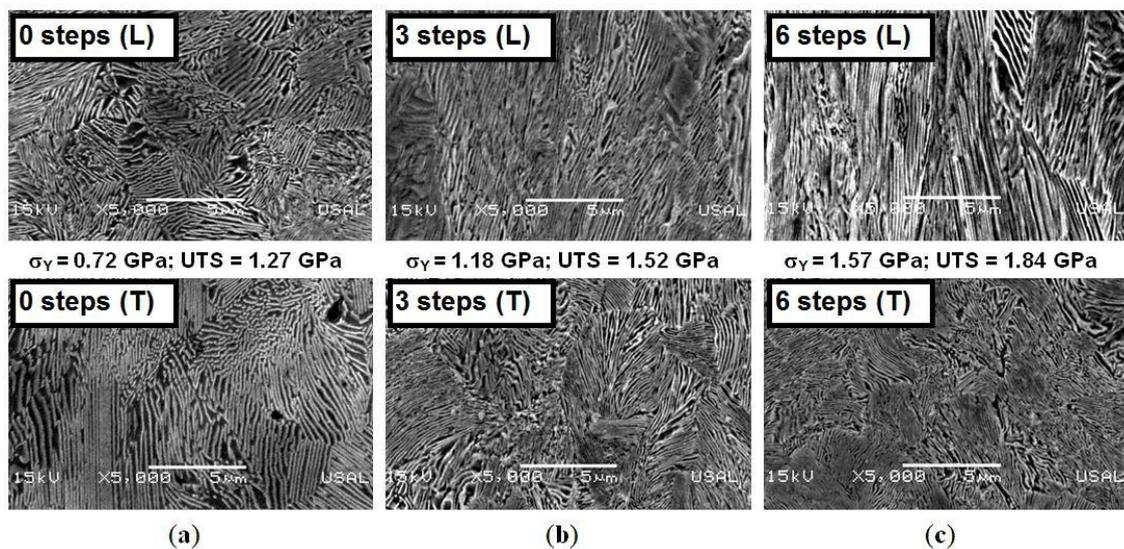
**Figure 1.** Micrographs of longitudinal (L) and transverse (T) sections of steels at different levels of cold drawing: (a) 0 steps, hot rolled bar; (b) 3 steps; (c) 6 steps, prestressing steel.
