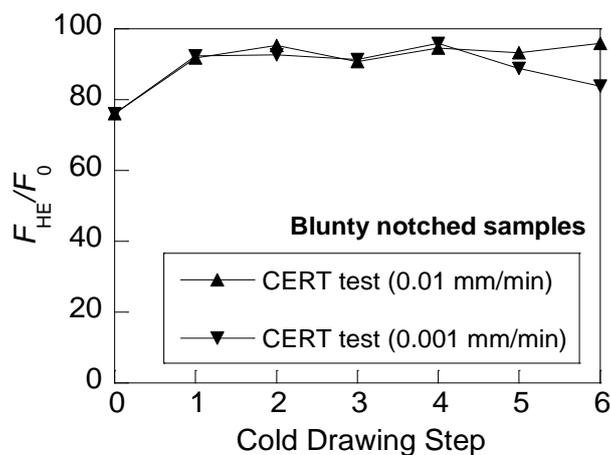
**Figure 8.** Variation with the cold drawing degree of the hydrogen embrittlement (HE) susceptibility of the progressively drawn steels for the two loading rates.
