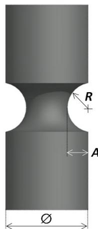
**Figure 2.** Round notched geometry used in the tests.
