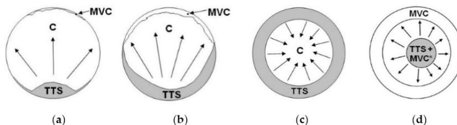
**Figure 7.** Schemes of the different models of micro-fracture map (MFM) in bluntly-notched samples of pearlitic steel under hydrogen embrittlement (HE) environmental conditions: (a) model I; (b) model II; (c) model III; (d) model IV.
