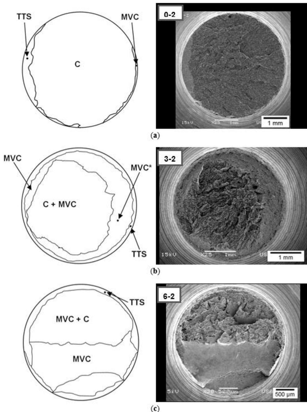
**Figure 5.** Micro-fracture maps (MFMs) for high loading rate (crosshead speed type 2 of 0.01 mm/min): (a) hot rolled steel (base material that is not cold drawn at all); (b) three drawing steps; (c) six drawing steps (heavily-drawn commercial prestressing steel).
