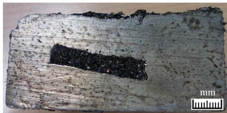
**Figure 9.** Central aluminium core covered with AM60B.
