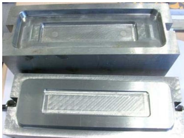
**Figure 3.** Metallic die to produce Aluminium foams with Alulight.
