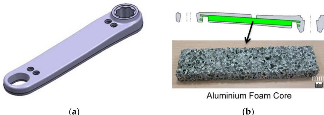
**Figure 2.** (a) 3D rod design; and (b) detail of the placement and example of an aluminium foam core.
