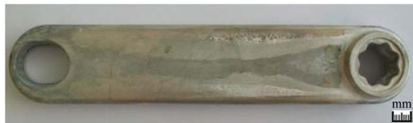
**Figure 17.** Rod made by magnesium HPDC with the internal core of aluminium foam.
