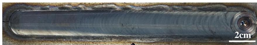
**Figure 1.** Appearance of the friction stir welding (FSW) joint.
