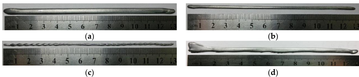
Figure 3. Various forming morphology with different combinations of process parameters. (a) Melt flowing. (b) Excellent formation. (c) Incomplete fusion. (d) Uncontrolled area.
