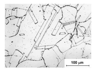
**Figure 2.** Microstructure of the 316L steel after solution annealing by regime 1050  $^{\circ}C/1$  h/water and stabilization annealing by regime 850  $^{\circ}C/4$  h/water.
