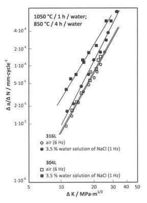
Figure 6. Kinetics of fatigue crack growth for 304L and 316L steels after stabilization annealing.
