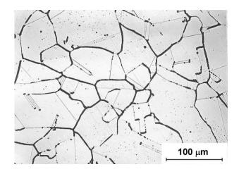
**Figure 3.** Microstructure of 316L steel after solution annealing by regime 1050  $^{\circ}C/1$  h/water and sensitization annealing by regime 600  $^{\circ}C/24$  h/water.
