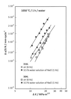
Figure 5. Kinetics of fatigue crack growth for 304L and 316L steels after solution annealing.
