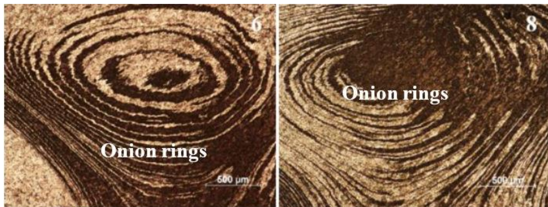
Figure 4. Nugget zone structures consisting of onion rings.
