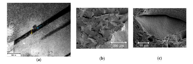
**Figure 16.** The 18Cr-10Ni-Ti steel in-service WWER irradiated to 5.2 dpa after tensile test at RT: (a) microstructure below fracture showing twins (yellow arrow) and strain martensite needles (blue arrow) [6]; Copyright 2017 by The Minerals, Metals & Materials Society. Used with permission; (b) fracture surface showing mix of dimples, secondary cracks and TG facets and (c) detail of the facet.
