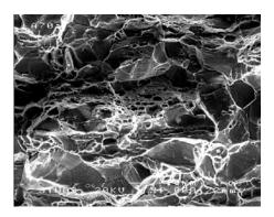
**Figure 6.** IG and ductile dimpled fracture of pin-loading tension specimen of a flux thimble tube (FTT), made from cold drawn A316, irradiation to 65 dpa in a PWR; fracture toughness test in air at room temperature [20]. Reproduced with the courtesy of A. Jenssen and Société Française d'Énergie Nucléaire (SFEN).
