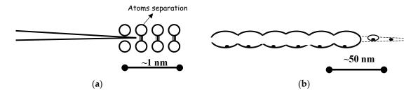
**Figure 1.** Schematic types of macro brittle intergranular fracture according [3]: (a) Atomically brittle intergranular fracture—featureless facets observed for high resolution SEM or TEM replicas often associated with embrittling segregation; (b) Nano-scale dimpled intergranular fracture—very shallow dimples—sometimes not resolved by SEM: can occur due to the micro void coalescence (MVC) process in the very narrow soft zone adjacent to grain boundary.
