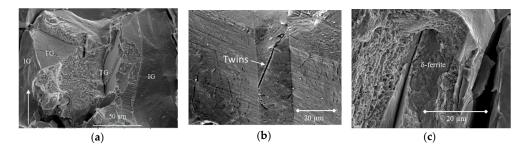
Figure 7. Fracture modes of the 2.4 dpa irradiated 18Cr-10Ni-Ti CT specimen if broken to open in nitrogen vapor at about  $-100\,^{\circ}$ C; arrow indicates the crack growth direction [3]: (a) Mixed IG with transgranular (TG) fracture connected by bridges of cleavage and ductile shear; (b) Twinning on grain boundary; (c) Fracture around a large δ-ferrite particle showing cleavage of the particle and secondary cracks close to ductile ridges.
