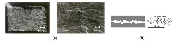
**Figure 13.** Quasi-cleavage of (a) specimen of 20%CW A316 (EBR-II, 460 °C, 78 dpa, 3–8% of void swelling) after tensile test at RT. Detail in right showing many fine voids. Adapted and modified according [31] with courtesy of F. A. Garner. (b) Scheme of the Quasi-cleavage fracture mechanisms—TG fracture owing cleavage rupture of bridges linking up micro-scale voids emphasizing that they are not deformed.
