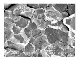
**Figure 5.** IG fracture of thin tensile specimens from the wide range neutron monitor guide tube of A304 steel irradiated in BWR to ~80 dpa and tensile tested at room temperature [19]. Reproduced with the courtesy of A. Jenssen and Société Française d'Énergie Nucléaire (SFEN).
