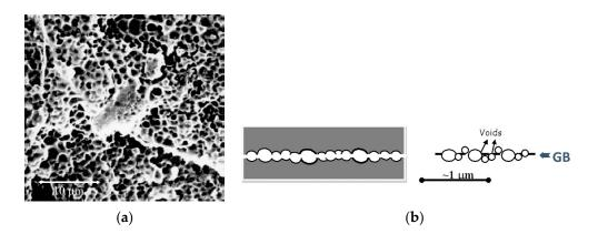
**Figure 14.** The fracture of the steel containing a higher than 15% void swelling at temperature  $T_t \approx T_{ir}$ : (a) 18Cr-10Ni-Ti ASS irradiated at BOR-60 to 72 dpa with 26% void swelling; after tensile test at 450–550 °C. Reproduced from [35] with courtesy of V. S. Neustroev. Elsevier reuse license has been granted. (b) Scheme of the fracture mechanism emphasizing that the void boundaries are deformed by creep and linked up.
