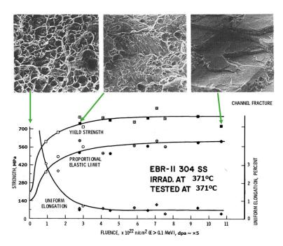
**Figure 10.** Effect of irradiation fluence on the yield strength and the uniform elongation of annealed 304 austenitic stainless steel (ASS) showing changing fracture appearance owing to increased plastic flow localization [30]. Note the channel fracture at ~54 dpa. Adapted and modified according [31] with courtesy of F. A. Garner.
