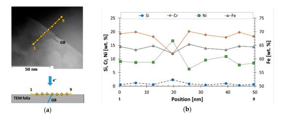
**Figure 3.** Scanning TEM Energy-dispersive X-ray spectroscopy (EDS) point analyses (from 1 to 9) in a marked line across a high-angle grain boundary of in-service irradiated 18Cr-10Ni-Ti of Russian PWR (WWER) RCI (5.2 dpa): (a) schematic showing position of the grain boundary (GB) in the TEM folia; (b) Depleted Cr and enriched Ni, Si was observed [6]. Copyright 2018 by The Minerals, Metals & Materials Society. Used with permission.
