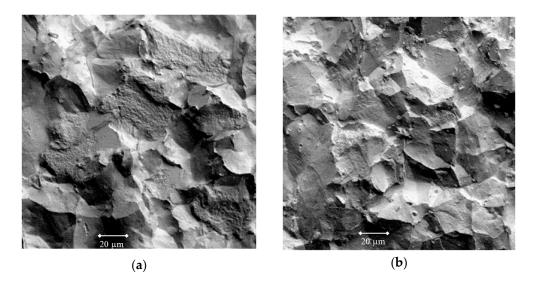
**Figure 12.** Fracture appearance of 18Cr-10Ni-Ti steel specimens irradiated at BOR-60 at 400–450 °C to 49 dpa (3–13% void swelling); showing IG and channel facets after tensile tests at: (a) 20 °C; (b) 290 °C [34]. Reproduced with courtesy of V. S. Neustroev. Copyright 2009 by The American Society of Mechanical Engineers (ASME). Acknowledgment to use with the permission.
