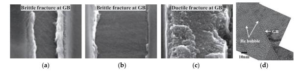
**Figure 17.** Unique SEM micrographs of grain boundary (GB) fracture of micro-tensile specimens of He-ion irradiated 15%CW316L, in a 45° perspective view: (a) 2% He; (b) 10% He; (c) 10% He post-irradiation annealed at 923K; (d) 6% He [18]. Reproduced with courtesy of K. Fukuya. Elsevier reuse license has been granted.
