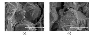
**Figure 8.** Complex brittle IG and TG fractures of the 5.2 dpa irradiated 18Cr-10Ni-Ti CT specimen if broken to open in nitrogen vapor at about  $-100\,^{\circ}$ C; arrows indicate the crack growth direction: (a) one specimen; (b) second specimen [3].
