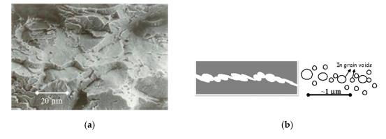
**Figure 11.** Example of channel fracture of: (a) 20%CW A316 irradiated at 385 °C to ~64 dpa in EBR-II and tensile tested by  $6 \times 10^{-4} \text{ s}^{-1}$  at 205 °C. Adapted and modified according [31] with courtesy of F. A. Garner. The material exhibited ~3–8% of void swelling. Courtesy of F. A. Garner [31]; (b) Scheme of the TG channel fracture owing shear of bridges linking up the voids according to the TEM image in [33].
