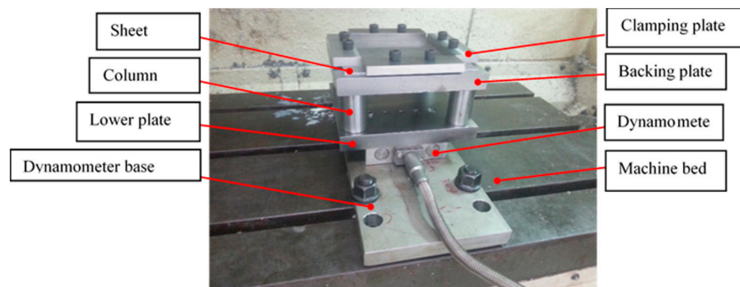
Figure 4. The forming jig with dynamometer.
