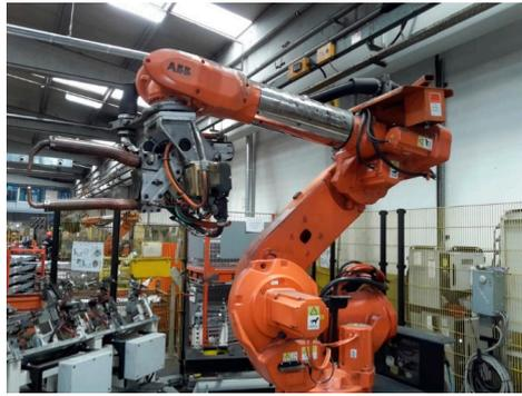
**Figure 4.** The medium-frequency direct current (MFDC) resistance spot-welding (RSW) machine connected to the ABB robot arm used in this investigation.
