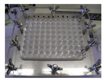
**Figure 1.** High-throughput corrosion inhibition rig consisting of a 10-mm-thick polycarbonate clamped to a 10-mm-thick block of polydimethylsiloxane rubber, an abraded plate of alloy, and a 5-mm-thick metal baseplate. The polycarbonate and polydimethylsiloxane sheets have a  $8 \times 11$  grid of holes for test solutions 6 mm in diameter. Used with permission from Winkler et al. [1].
