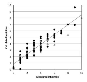
**Figure 2.** Quantitative prediction of corrosion inhibitory properties of organic compounds for aerospace alloys AA-2024 generated using molecular descriptors (not derived from quantum mechanical calculations). Inhibition is scaled between 0 (no inhibition) and 10 (highest inhibition). The circles represent the performance of the model in predicting training set, and the triangles represent the performance of the model in predicting the test set. Used with permission from Winkler et al. [1].
