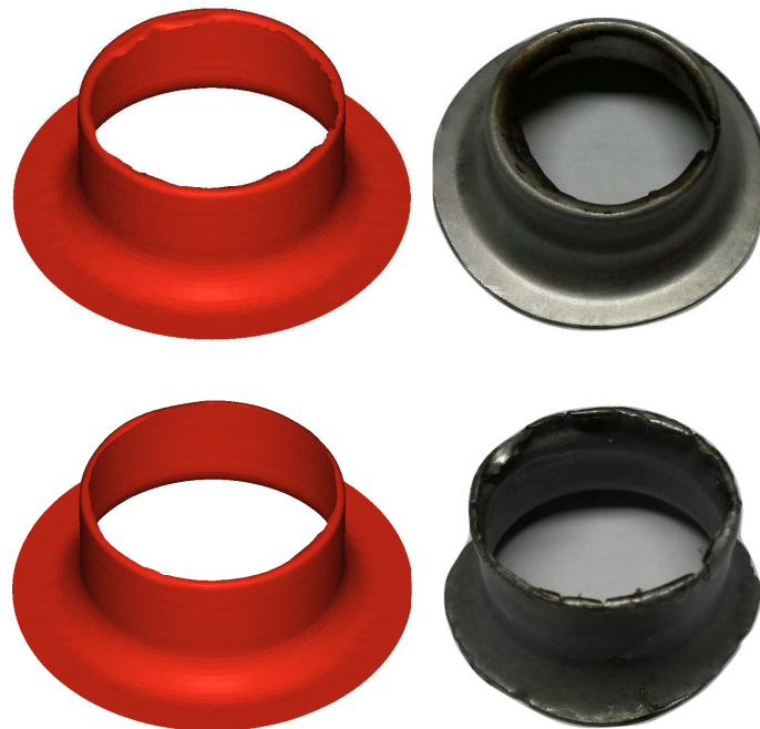
Figure 14. Damage caused by the high-pressure load profile (130% of experimental load). Snapshots of the fully damaged samples: numerical simulations ( left ) and experiments ( right ).
