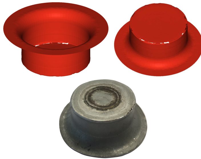
Figure 13. Damage occurring due to scaled load (110% of the optimum experimental load). Minor damage was observed along the corner. Comparison of the snapshots obtained in the numerical simulations ( top ) and experiments ( bottom ).
