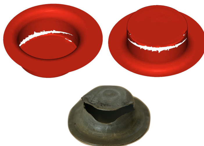
Figure 16. Initial misalignment of 3 mm between the blank and the die. Fractured workpieces in numerical simulations ( top ) and specimen in the experiment ( bottom ).
