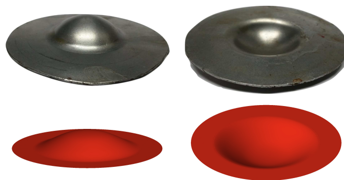
Figure 12. Comparison of the final shape obtained in the experiments ( top ) and numerical simulations ( bottom ) due to low-pressure load (60% of the optimum experimental load).
