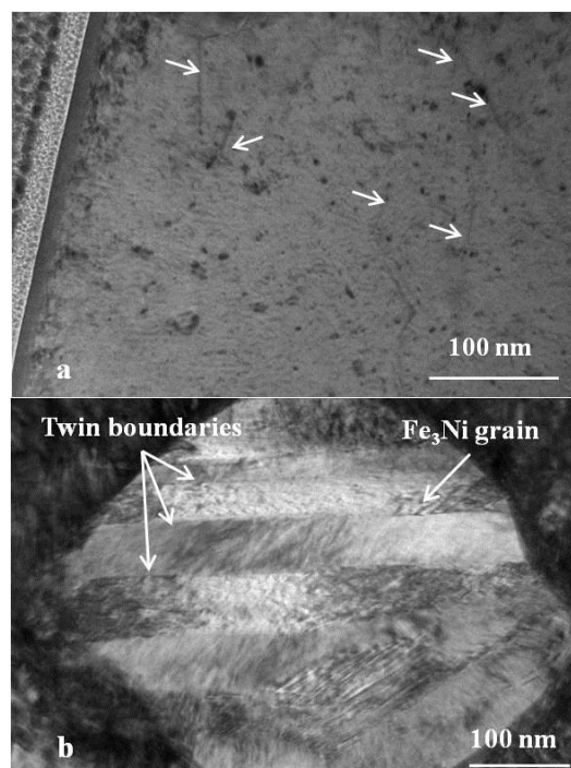
Figure 9. Crystal lattice defects in the hot-pressed Fe–Co–Ni samples made from the mixtures subjected to MA for 15 min: dislocations (a) (shown with arrows) and twin boundaries (b).
