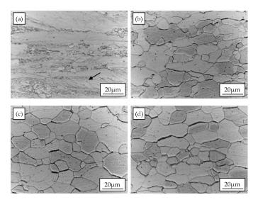
**Figure 2.** Optical micrographs of experimental steel batch annealed at different temperatures (**a**) 580 °C; (**b**) 630 °C; (**c**) 680 °C; (**d**) 730 °C.
