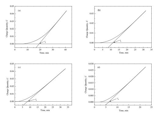
**Figure 8.** Hydrogen permeation curves (charge quantity vs. time curves) of ultra-low carbon enamel steel annealed at different temperatures (a) 580 °C; (b) 630 °C; (c) 680 °C; (d) 730 °C.
