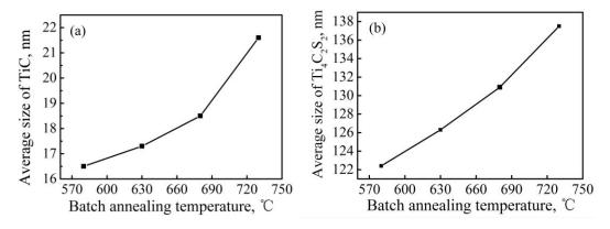
**Figure 6.** Effect of the batch annealing temperature on the average sizes of TiC (a) and Ti<sub>4</sub>C<sub>2</sub>S<sub>2</sub> (b).
