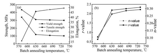
**Figure 7.** Relationship between the mechanical properties and batch annealing temperature of ultra-low carbon enamel steel. (a) Strength and Elongtation; (b) n and r value
