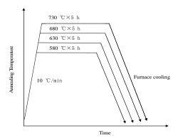
Figure 1. Schematic of the batch annealing process of ultra-low carbon enamel steel.
