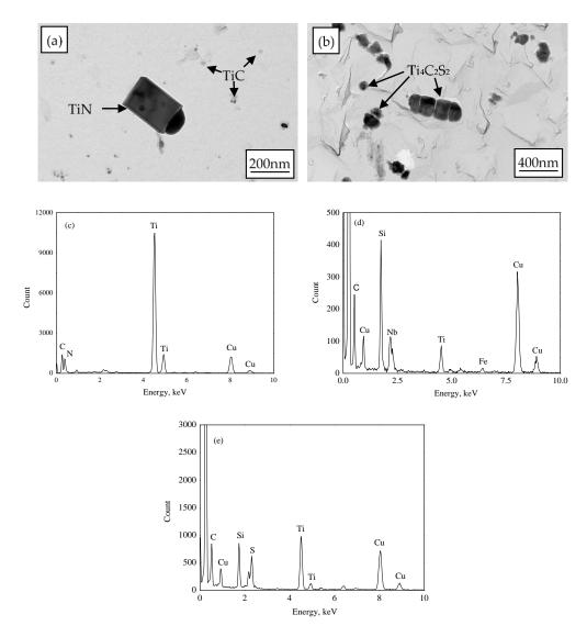
**Figure 4.** Transmission electron microscope (TEM) micrographs showing precipitates in experimental steel (a) TiN and TiC particles; (b)  $Ti_4C_2S_2$  particles; (c) Energy dispersive spectrometer (EDS) spectrum of TiN; (d) EDS spectrum of TiC; (e) EDS spectrum of  $Ti_4C_2S_2$ .
