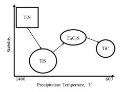
**Figure 5.** Schematic illustration of the stability of various Ti compounds in Interstitial-Free (IF) steels as a function of the precipitation temperature.
