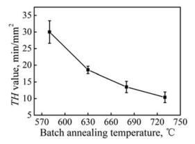
**Figure 9.** Effect of the batch annealing temperature on the *TH* value of ultra-low carbon enamel steel.
