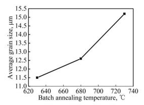
**Figure 3.** Effect of the batch annealing temperature on the average size of ferrite grain of ultra-low carbon enamel steel.
