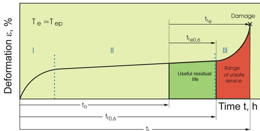
Figure 1. Schematic approach of the definition of residual and disposable durability.
